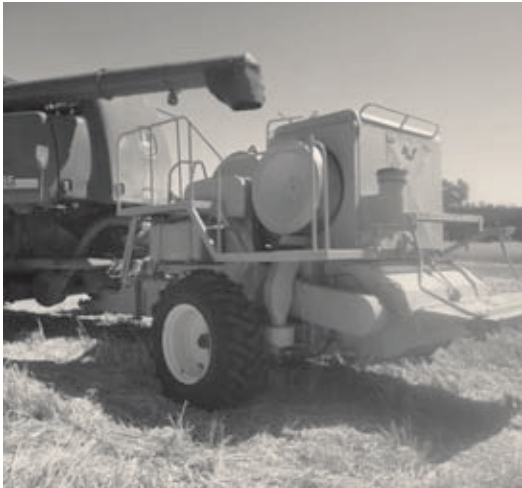
The Harrington Weed Seed Destructor is not a 'silver bullet' but crushes weed seeds at harvest, allowing growers to use non-chemical weed control as part of the integrated weed management package. Photo: Nicole Baxter, CORTEXT
