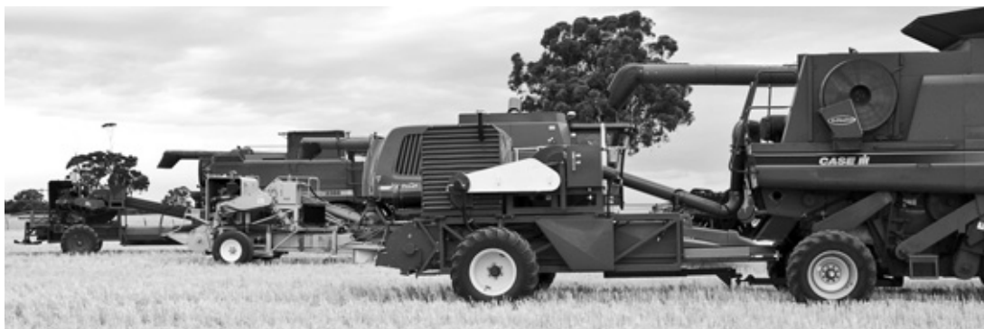
The three prototypes of the Harrington Weed Seed Destructor on the Harringtons' farm at Wagin, WA, during harvest 2010.
