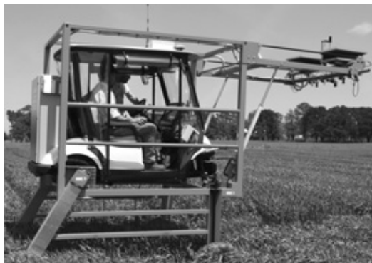
The Phenomobile developed by CSIRO and equipped with multispectral cameras and other apparatus to capture a wealth of physiological data in experimental plots at the managed environment facilities. Photo: CSIRO
