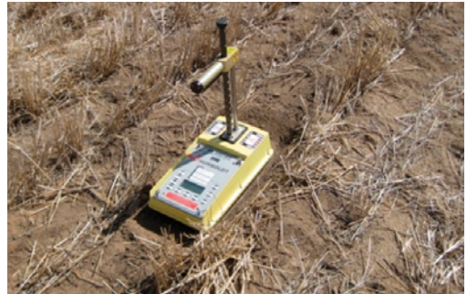
A neutron density meter allows researchers to assess soil bulk density within minutes. Photo: CSIRO Land and Water
