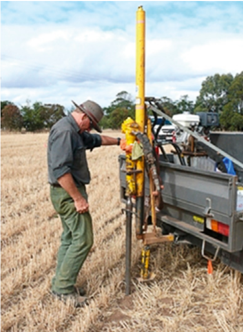
A researcher uses a vehicle-mounted hydraulic soil sampler to obtain cores for testing soil carbon. Photo: CSIRO Land and Water
