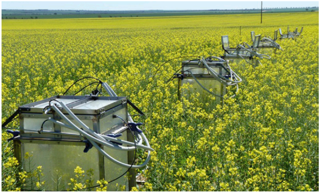
Gas collection chambers measure nitrous oxide in a canola crop at a trial site at Buntine, Western Australia. Photo: GRDC
