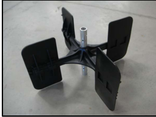
Figure 42. Amphibious Vehicle Paddle Wheel
