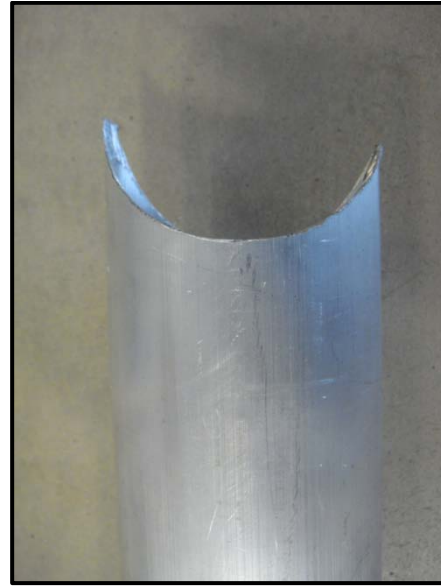
Figure 20. Tube with Fish Mouth Cut
