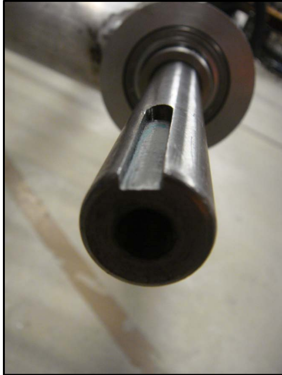
Figure 23. Drilled and Taped End of the Front Axle
