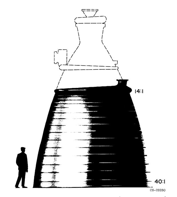
Figure 6. - M-1 Rocket Engine Project - Nozzle Extension (Area Ratio 14:1 to 40:1).
