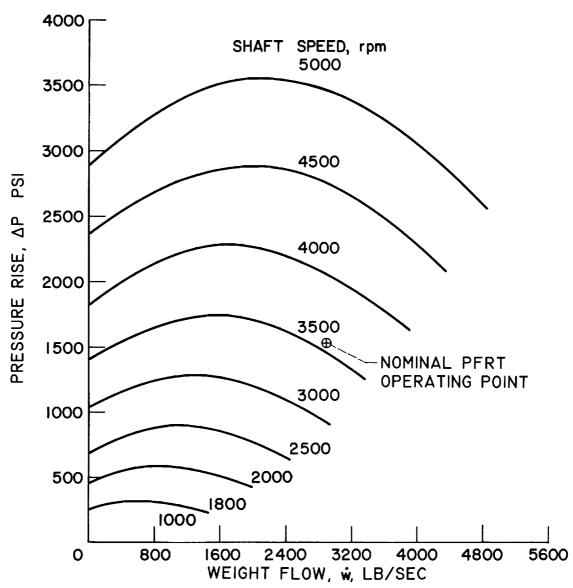
Figure 11. - M-1 Rocket Engine Project - Predicted Oxidizer Pump Performance.
