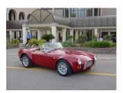
A new model was developed, the AC MKV, composite bodied on the original design steel ladder chassis and fitted with a Ford 5 L 340 hp fuel injected engine and 5 speed manual transmission. Production of the new AC MKV commenced in 2004 and ceased in 2007.
