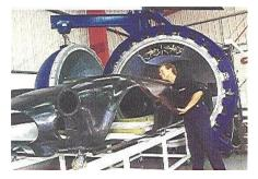
One of the main problems with composite panels is maintaining the shut gaps and surface integrity, carbon fibre is far more stable than glass fiber. As a result of welding of the separate panels the aluminium body becomes a one piece structure, the carbon fiber continued the trend, thus ensuring shut gap control and the overall quality was maintained.
