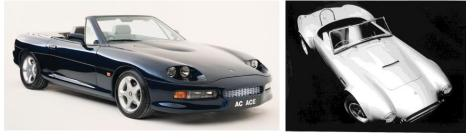
resurrecting the ACE name. It was a modern version of the AC Ace with air conditioning, electric windows and a new stainless steel chassis with an aluminium body.
