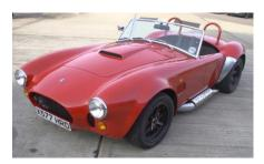
To create an evolution of the legendary MKIII 427 Cobra the company linked with Lotus mating their new 3.5 L V8 engine with a 6 speed transmission, the AC 212 was born delivering 350 hp in a 900 kg car. Unfortunately Lotus had to cease production of the engine so only 2- 212's were built in the end
