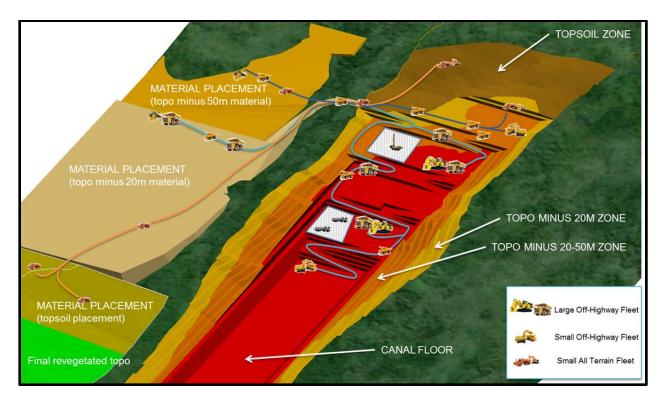
Figure 4.6-8: Excavated Material Placement
