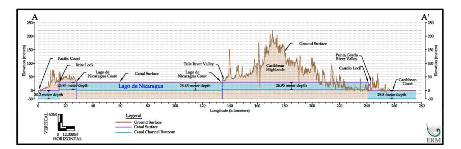
Figure 2-2: Canal Cross Section (200 Vertical Exaggeration)
