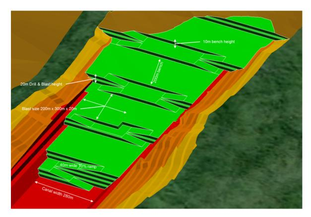
Figure 4.6-6: Graphic of Benched Excavation within Canal Footprint
