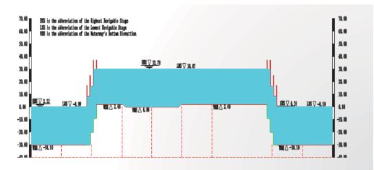
Figure 3.1-3: Schematics of Water Level Change
