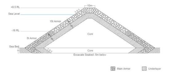
Figure 3.1-15: Typical Cross Section of the Breakwater Structures
