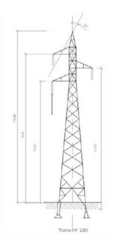
Figure 3.3-4: Proposed Electrical Transmission Towers
