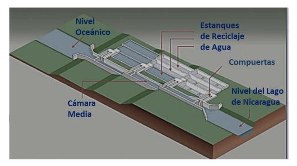
Figure 3.1-4: Concept Lock with 3 Chambers and 9 Water Saving Basins
