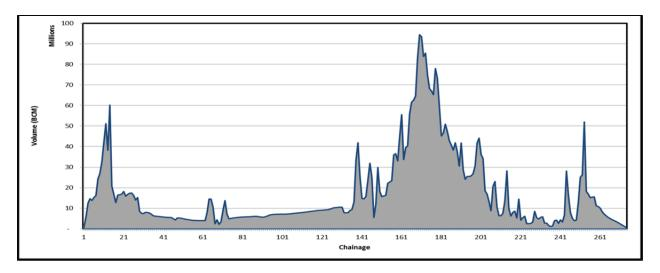
Figure 3.1-9: Canal Excavation Volumes by Station
