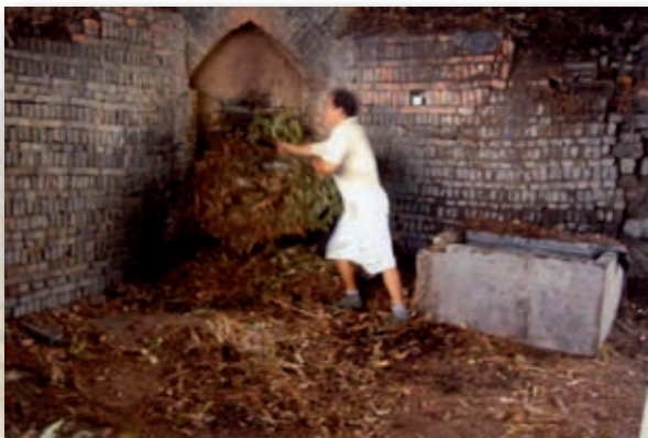
Firing bricks using traditional methods (Provided by Lam Ancestral Hall)
