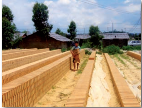
Drying bricks under the sun (Provided by Lam Ancestral Hall)
