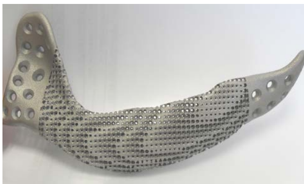
Finished jaw bone in Ti64 powder
