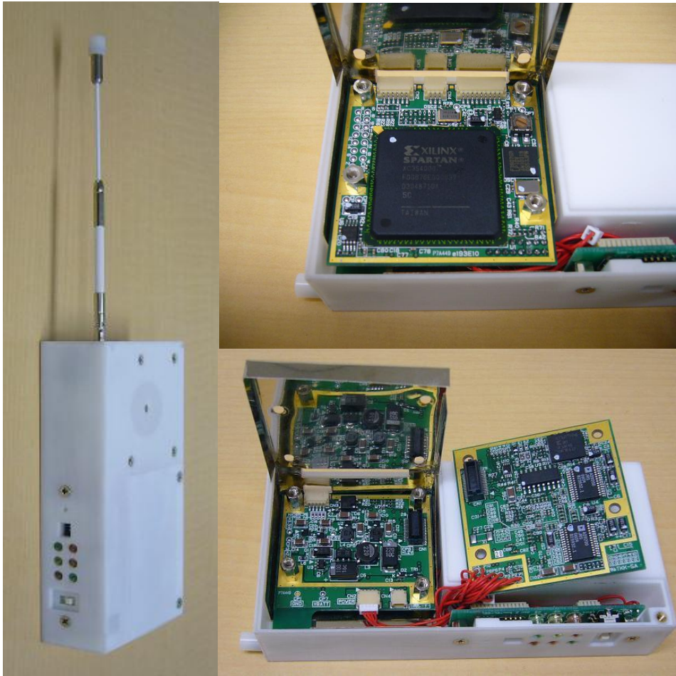
Small prototype receiver that detects the activation flag for alert broadcasting
