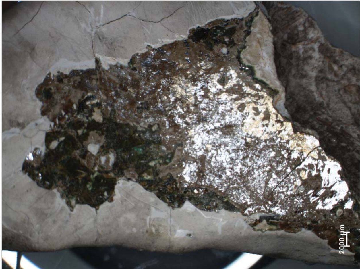
Figure 7.7. Paint exposure on fireplace flame, revealing layers of green, metallic leaf and bronzing powder, 7.1x mag, reflected light (L.Drapala, 2010).
