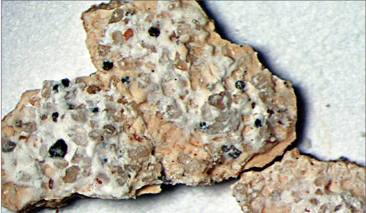
Figure 6.3. Macro photos of small detached sections of the paint that show the sandy finish plaster selectively attached to the back side of the gesso (J. Zucker, 2007).
