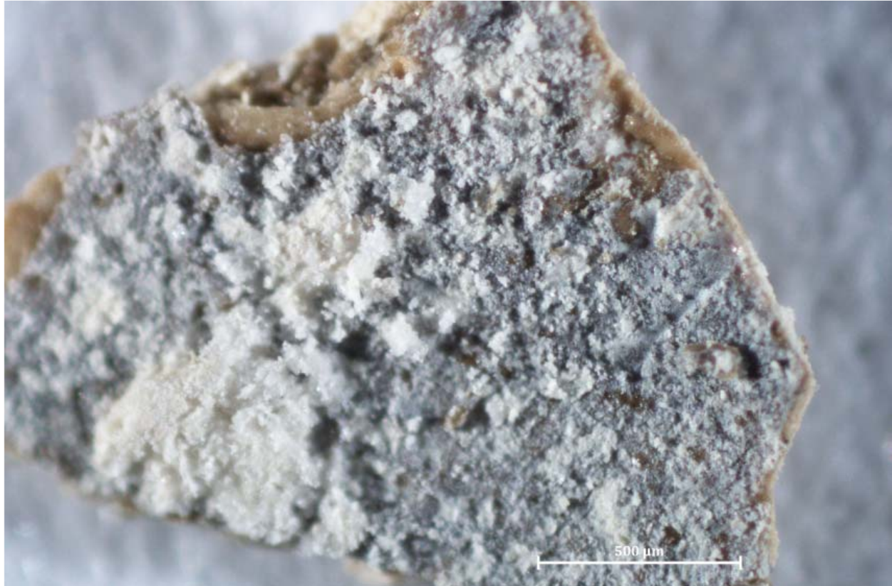
Figure 1.1. WHITP4_01 paint flake under 5x magnification, showing original silvery matte paint, loosely bound to its white preparatory layer. (L. Drapala, 2010).
