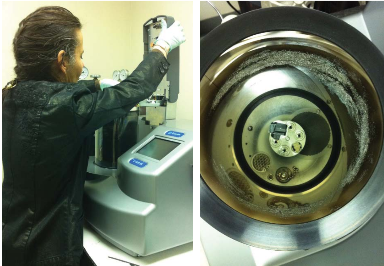
Figure 7.10. Lolita Rotkina preparing samples for SEM-EDS with carbon coating (L.Drapala, 2011).
