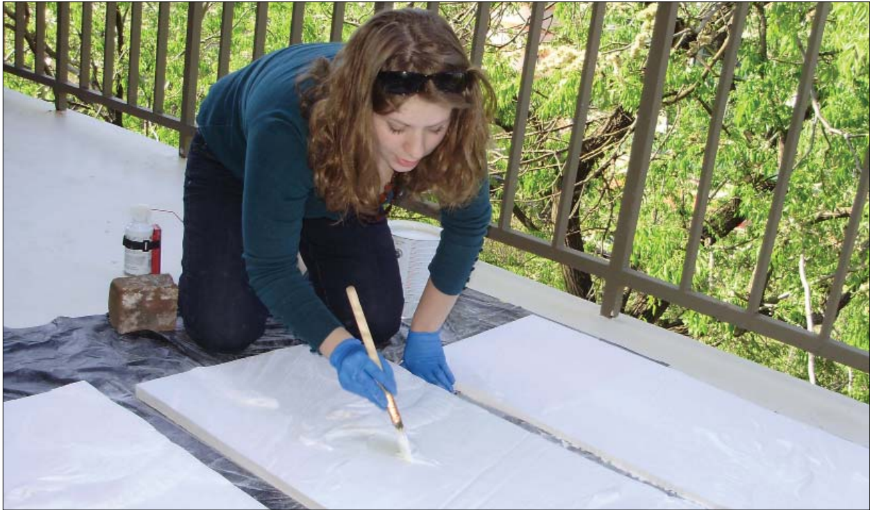
Figure 8.6. Lauren Drapala applying B-I-N Shellac Base to each plaster mold (Y. Hernandez, 2010).
