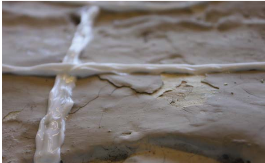
Figure 2.5. Example of consolidation treatment. The top image shows a portion of flaking paint, prior to treatment. The second image shows the flake after Acryloid B72 had been applied through syringe, and braced with cotton swabs. The bottom image shows the flake, fixed to the surface (2011).
