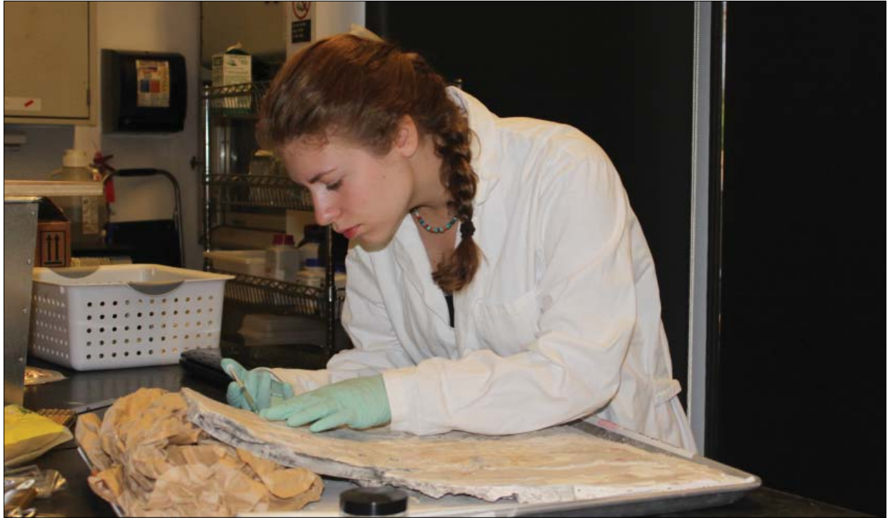
Figure 4.4. Consolidating the mock-up portion of the panel with 10% Aquazol in water (2011).
