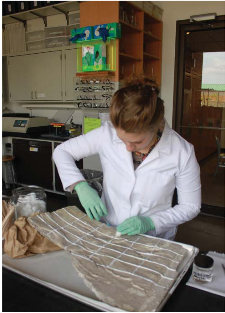
Figure 2.4. Lauren Drapala applying consolidant to panel through needle and syringe (2011).
