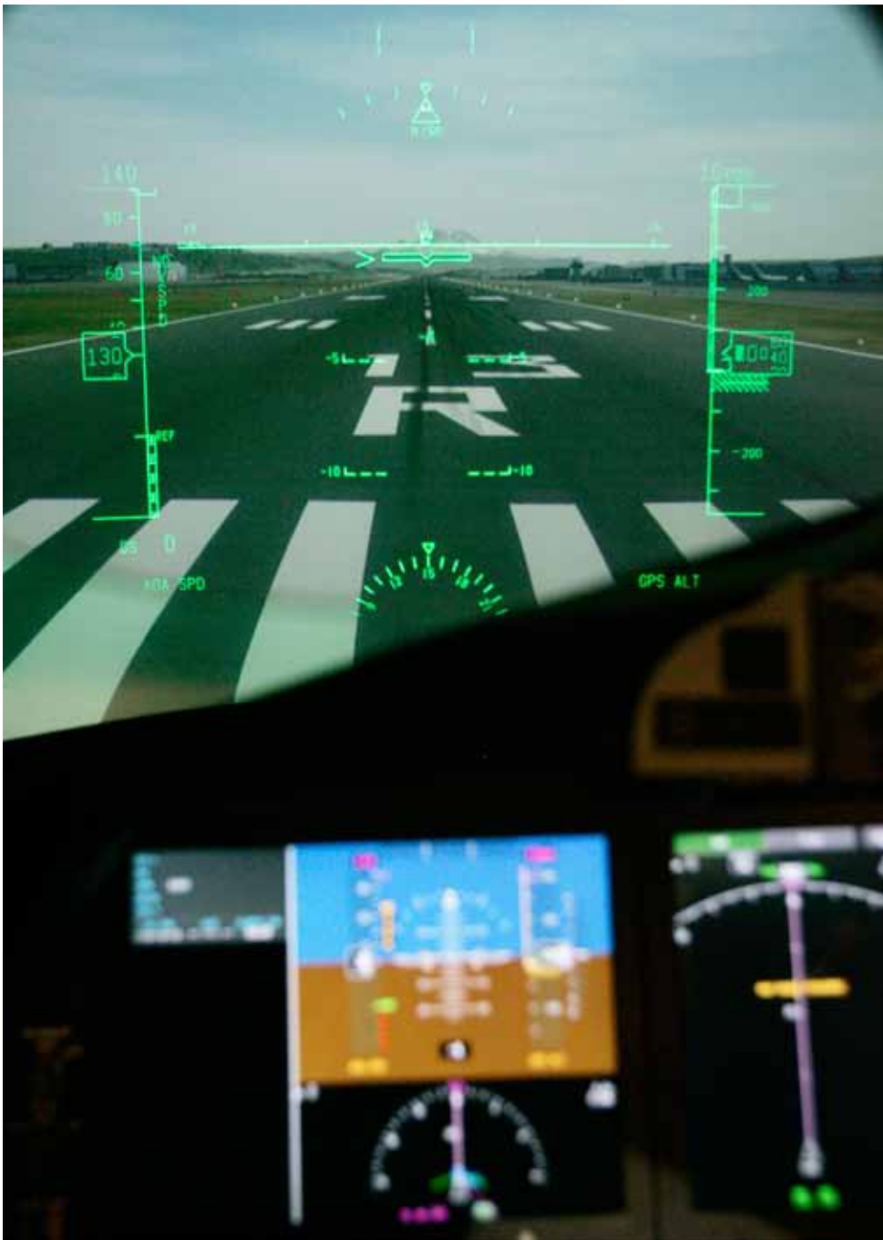
PILOT'S VIEW: Aircraft flight information is shown on a heads-up display in the Boeing 787 Dreamliner Engineering flight deck simulator during a media tour of Boeing Co. engineering labs in Seattle, Washington, May 22, 2007. REUTERS/ROBERT SORBO
