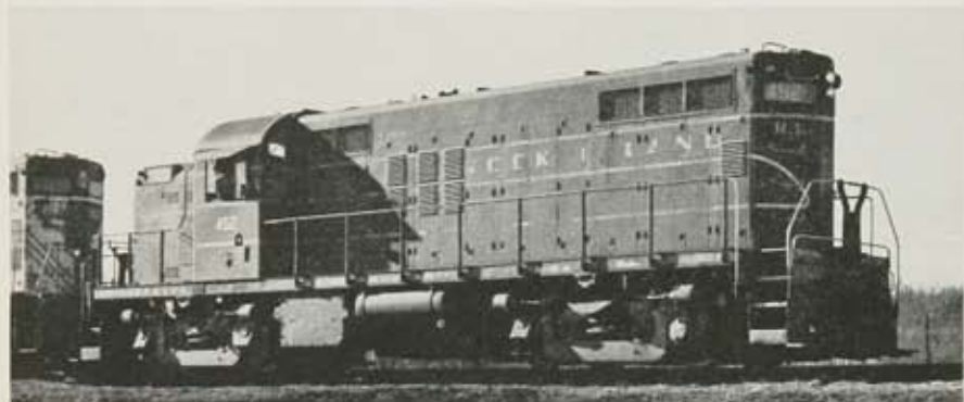
SWITCHING at Howe, Okla., is a former Alco 1500 h.p. RS-2, which was re-engined at La Grange and, in the process, fitted with a Geep long hood over its 567-series V-16 engine.
