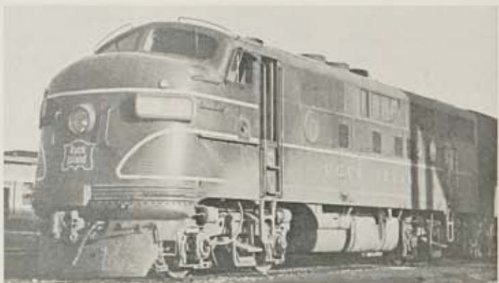
F249 OR had top headlight removed during a shopping, thus creating a unique variant of Electro-Motive's famous bulldog nose design.
