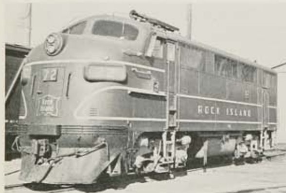
WOULD you believe it?—the 72 was an FT, disguised by large number boards, Mars light, and absence of portholes.
