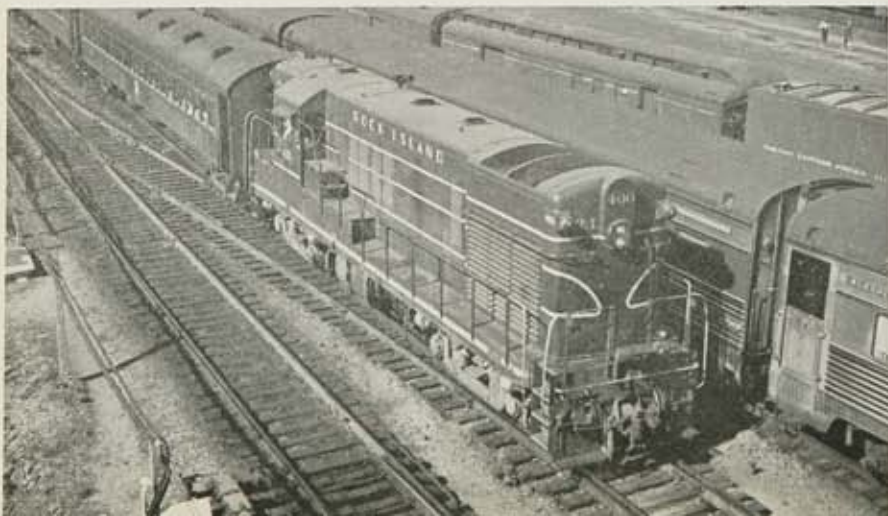
HERE'S Christine, the sole surviving example of Alco's prewar, Otto Kuhler-styled DL-109 passenger unit. She acquired her nickname and peaked roof when re-powered by Electro-Motive. GM 567's also chant away inside Rock Island's only two Fairbanks-Morse units (below) — road-switchers 400 and 401. Twin stacks are sole hint of foreign power plants.
