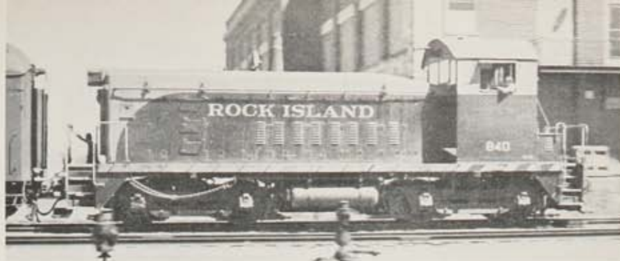
ROCK ISLAND acquired a pair of EMD SW8 yard goats with the purchase of a Texas short line — Wichita Falls & Southern — in 1954. Renumbered 840 switches in WF&S colors.
