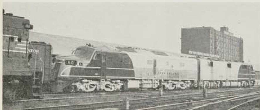
HERE'S Christine, the sole surviving example of Alco's prewar, Otto Kuhler-styled DL-109 passenger unit. She acquired her nickname and peaked roof when re-powered by Electro-Motive. GM 567's also chant away inside Rock Island's only two Fairbanks-Morse units (below) — road-switchers 400 and 401. Twin stacks are sole hint of foreign power plants.
