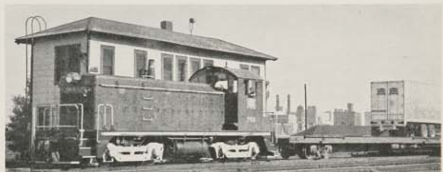
DEMISE of the New York, Ontario & Western in 1957 placed 1000 h.p. EMD NW2's 795-797 (ex-O&W 111-113) on the Rock Island. Sample 796 leads piggyback over an IC diamond.
