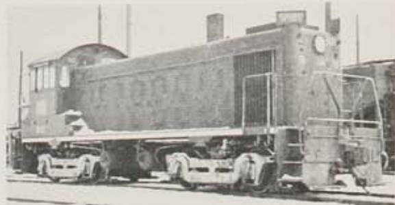
ONE of only two Lima 800 h.p. switchers built with a rear "step" containing battery box (above), the 801 was traded in on a GP35 this year. Ex-Rocky Mountain Rocket 751 (below) now rolls commuters in bi-level Budds.
