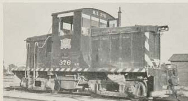
CENTER-CAB 44-tonner 376 is a mate of Davenport 351, the unit that pioneered one-man-operated locomotives before the war.
