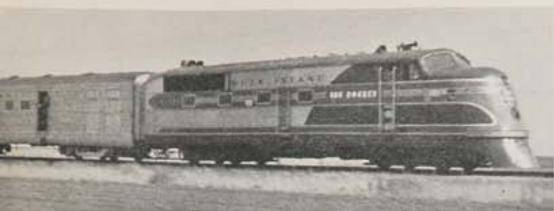
ONE of Rock Island's unique 1200 h.p. B-B EMD TA's speeds across Oklahoma with the Choctaw Rocket (above). Ex-Canadian National Whitcomb 1002 wears a protective shield while on lease to Big Rock Gravel at Little Rock. Firm later purchased the 75-ton Dominion diesel unit.
