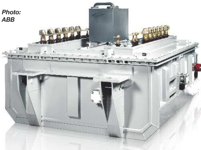
ABB's traction transformer for the IOREs has an aluminium housing. Its design power is 7,162 kVA, and it comprises four traction windings, two filters, one auxiliary reactor and two secondary harmonics filter reactors. It weighs 14 t and has losses of 260 kW. It was developed jointly by ABB and Bombardier's Oerlikon works in Switzerland.
