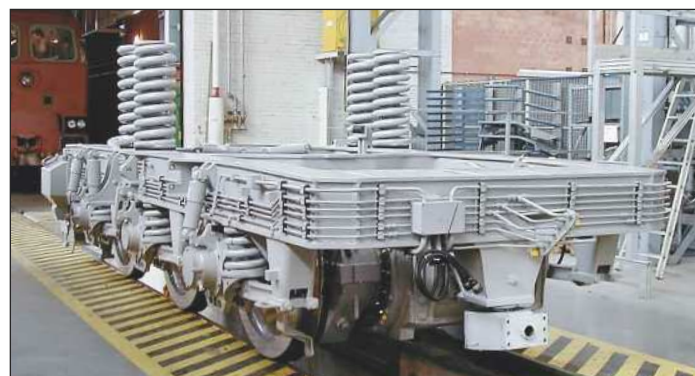
An IORE bogie, showing the massive derailment protection beam, photographed at Kassel on 11 May 2000 following delivery from the works at Siegen. Note the steel pipes and tubes on the outside of the bogie frames in the right-hand photo.
