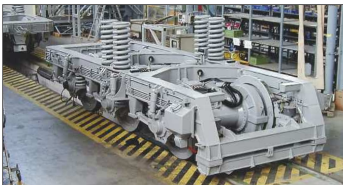
An IORE bogie, showing the massive derailment protection beam, photographed at Kassel on 11 May 2000 following delivery from the works at Siegen. Note the steel pipes and tubes on the outside of the bogie frames in the right-hand photo.
