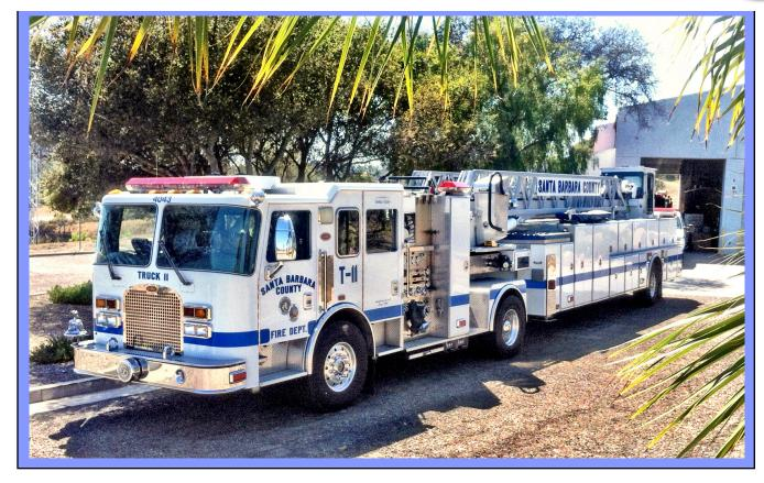
SBC has a KME tractor-drawn aerial which is located at Station 11 in the City of Goleta. The truck weighs 74 thousand pounds and has a 100' aerial ladder, which is piped with a nozzle at the tip of the ladder making it possible for an elevated stream of up to 1,250 GPM high above the fire. It's technical term is a Quint, which means it has a pump, water tank, aerial ladder and carries ground ladders and fire hose.
