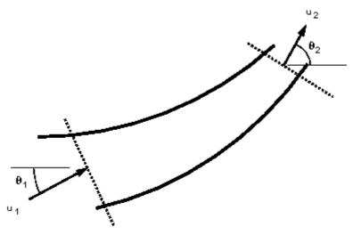
Two dimensional flow in a streamtube
