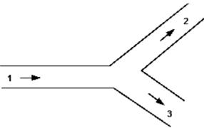
Total mass flow into the junction = Total mass flow out of the junction
