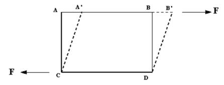
Shearing force, F, acting on a fluid element.
