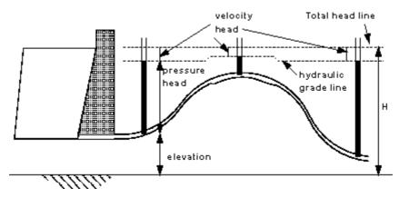
Piezometer levels and velocity heads with fluid flowing in varying diameter pipes
