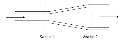
If the diameter at section 1 is  $d_1 = 30mm$  and at section 2  $d_2 = 40mm$  and the mean velocity at section 2 is  $u_2 = 3.0m/s$ . The velocity entering the diffuser is given by,
