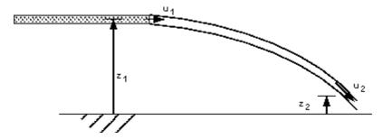
The Trajectory of a jet of water
