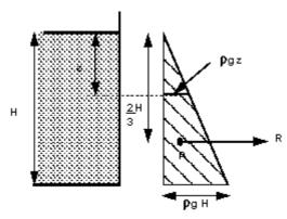
Pressure diagram for vertical wall.
