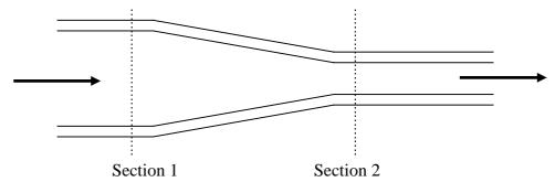
A liquid is flowing from left to right and the pipe is narrowing in the same direction. By the continuity principle, the mass flow rate must be the same at each section - the mass going into the pipe is equal to the mass going out of the pipe. So we can write:
