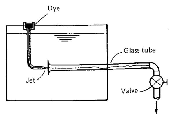
He used a tank arranged as above with a pipe taking water from the centre into which he injected a dye through a needle. After many experiments he saw that this expression
