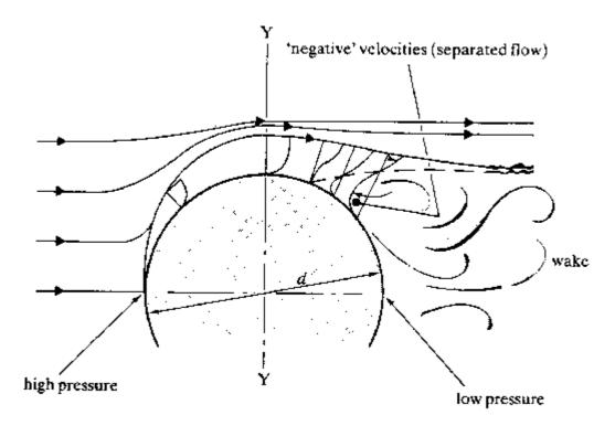
Looking at the figure above, the formation of the separation occurs as the fluid accelerates from the centre to get round the cylinder (it must accelerate as it has further to go than the surrounding fluid). It reaches a maximum at Y, where it also has also dropped in pressure. The adverse pressure gradient between here and the downstream side of the cylinder will cause the boundary layer separation if the flow is fast enough, (Re > 2.)
