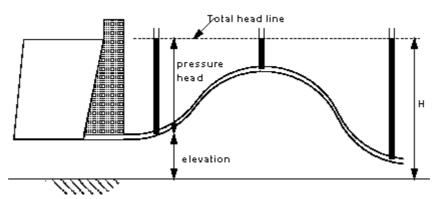
Piezometer levels with zero velocity
