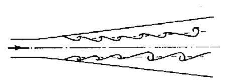
Increasing the angle of the diffuser increases the probability of boundary layer separation. In a Venturi meter it has been found that an angle of about 6° provides the optimum balance between length of meter and danger of boundary layer separation which would cause unacceptable pressure energy losses.
