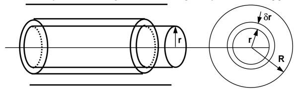
We are in equilibrium, so the shearing forces on the cylinder equal the pressure forces.
