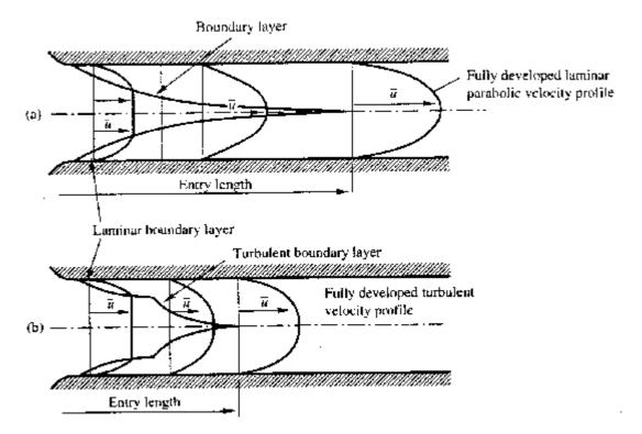
If we only have laminar flow the profile is parabolic – as proved in earlier lectures – as only the first part of the boundary layer growth diagram is used. So we get the top diagram in the above figure.
