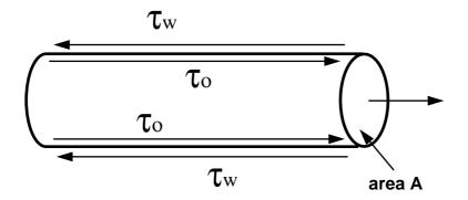
The pressure at the upstream end is p, and at the downstream end the pressure has fallen by  $\Delta p$  to  $(p-\Delta p)$ .
