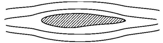
Streamlines around a wing shaped body
