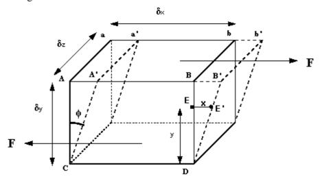
Fluid element under a shear force
