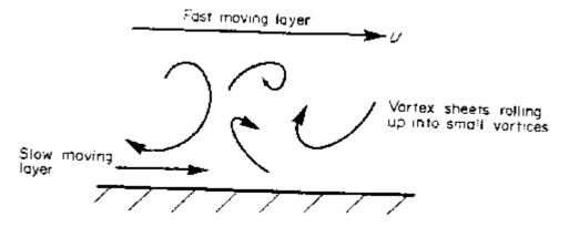
This causes the fluid motion to rapidly becomes turbulent. Fluid from the fast moving region moves to the slower zone transferring momentum and thus maintaining the fluid by the wall in motion. Conversely,
