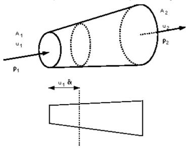
A streamtube in three and two-dimensions
