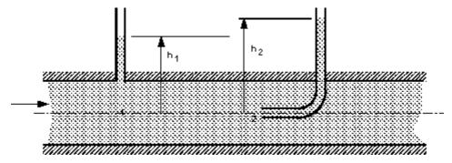
A Piezometer and a Pitot tube
