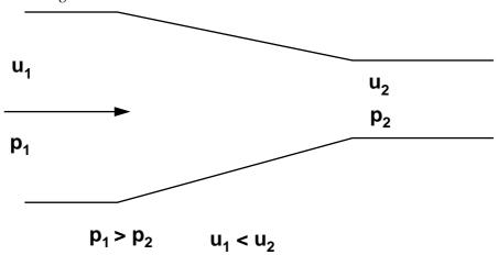
The accelerating fluid maintains the fluid close to the wall in motion. Hence the flow remains <u>stable</u> and turbulence <u>reduces</u>. Boundary layer separation <u>does not</u> occur.
