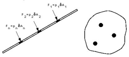
We can find the total or *resultant* force, R, on the plane by summing up all of the forces on the small elements i.e.
