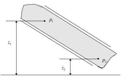
The pipe is filled with stationary fluid of density  $\rho$  has pressures  $p_1$  and  $p_2$  at levels  $z_1$  and  $z_2$ respectively. What is the pressure difference in terms of these levels?
