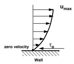
Looking at this two-dimensionally we get the above velocity profile from the wall to the centre of the flow.
