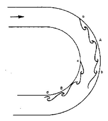
Two separation zones occur in bends as shown above. The pressure at b must be greater than at a as it must provide the required radial acceleration for the fluid to get round the bend. There is thus an adverse pressure gradient between a and b so separation may occur here.
