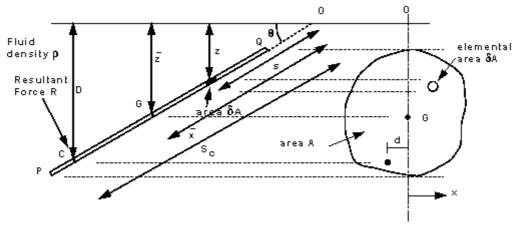
This plane surface is totally submerged in a liquid of density  $\rho$  and inclined at an angle of  $\theta$  to the horizontal. Taking pressure as zero at the surface and measuring down from the surface, the pressure on an element  $\delta A$ , submerged a distance z, is given by
