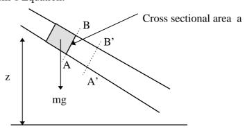
An element of fluid, as that in the figure above, has potential energy due to its height z above a datum and kinetic energy due to its velocity u. If the element has weight mg then
