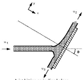
A jet hitting an inclined plane.
