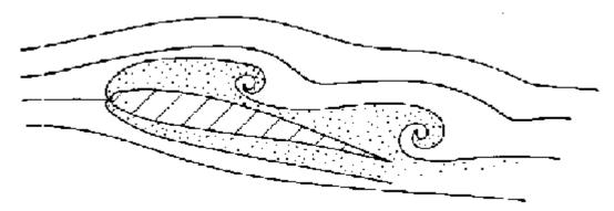
When stalling occurs, all, or most, of the 'suction' pressure is lost, and the plane will suddenly drop from the sky! The only solution to this is to put the plane into a dive to regain the boundary layer. A transverse lift force is then exerted on the wing which gives the pilot some control and allows the plane to be pulled out of the dive.
