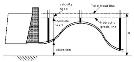
Piezometer levels when fluid is flowing
