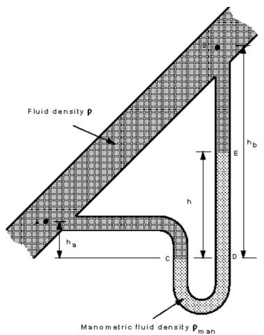
Pressure difference measurement by the "U"-Tube manometer
