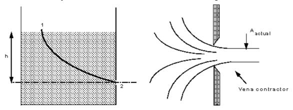
Tank and streamlines of flow out of the sharp edged orifice
