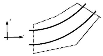
The control volume is draw in the above figure, with faces at the inlet and outlet of the bend and encompassing the pipe walls.
