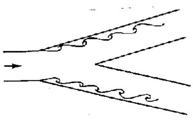
Downstream, away from the junction, the boundary layer reattaches and normal flow occurs i.e. the effect of the boundary layer separation is only local. Nevertheless fluid downstream of the junction will have lost energy.
