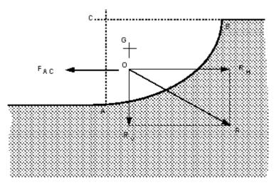
The calculation of the forces acting from the fluid below is very similar to when the fluid is above.
