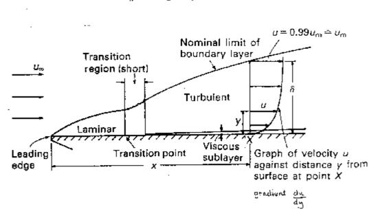
We define the thickness of this boundary layer as the distance from the wall to the point where the velocity is 99% of the "free stream" velocity, the velocity in the middle of the pipe or river.
