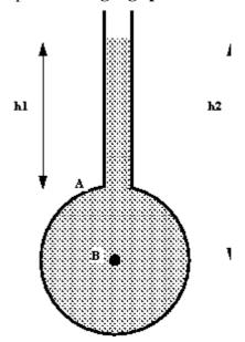
A simple piezometer tube manometer
