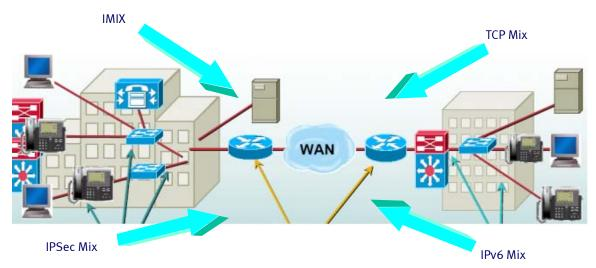
A realistic mixture of packet sizes will be classified into 4 different IMIX-oriented sets. For ease of data management and troubleshooting, the "simple" IMIX approach will be used in the first test. Once the throughout rate is determined, subsequent tests in the next section will expand upon an IMIX set and add frame sizes and random ranges.
