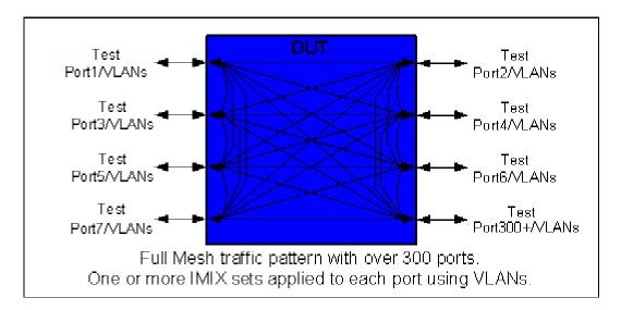
IMIX traffic may traverse multiple ports in many traffic patterns. Each port may emulate its own unique mix of Internet traffic. When applied to VLAN-tagged ports IMIX patterns emulate traffic from logical interfaces.
