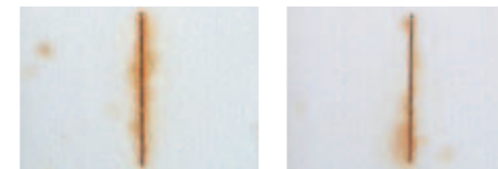
Modified epoxy resin anticorrosive coating 2 coats of 60µm (total thickness: 120µm) ESCO NB Mild H 1 coat of 120µm (total thickness: 120µm)
