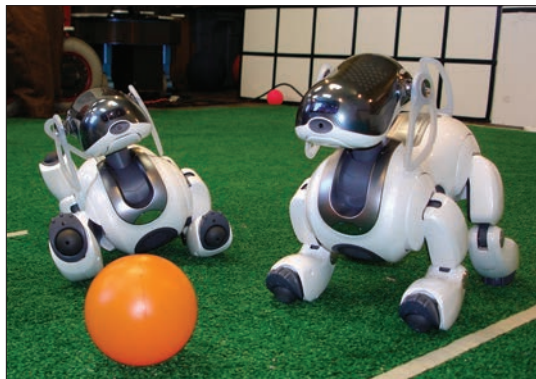
ABOVE Brown's two RoboCup teams will use the Sony Aibo. Teams of four dogs will compete against each other in a soccer match.
