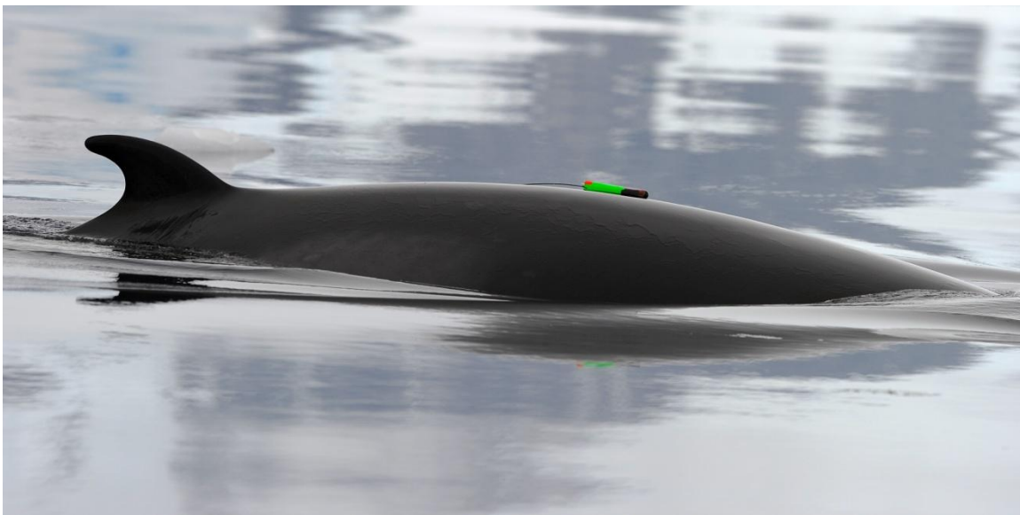
Image 1. Multi-sensor archival suction-cup tag (Acousonde) deployed on an Antarctic minke whale, Wilhelmina Bay, Antarctic Peninsula, February 2013. Tag sensors include pressure, temperature, 3-axis accelerometers and magnetometers, hydrophone, and VHF.
