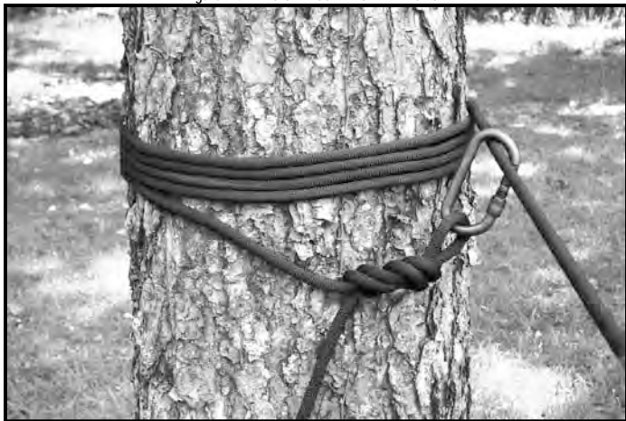
Figure 9-4. TENSIONLESS NATURAL ANCHOR
