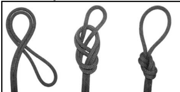
Figure 9-10. DOUBLE FIGURE 8 LOOP KNOT
