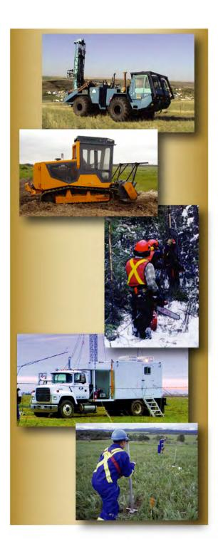
A seismic survey is a method of determining sub-surface information by analyzing sound waves originating from an energy source, which is typically either a small amount of explosive in a shot hole, drilled to depths up to about 60 feet / 20 metres or, vibrations generated from a series of "vibroseis" trucks.
