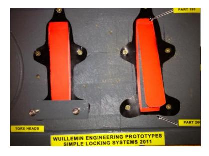
Fig 9.Design (a) hatch handle prevented from lifting upward - coded screws in place.
