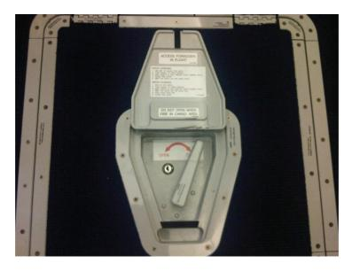
Fig 7. Airbus Hatch For Aft Cabin Flooring - locking handle in view (KC30 RAAF).
