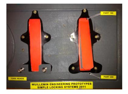
*Fig 10. Design (b) hatch handle with slotted plate in place – sideways movement frees handle.*
