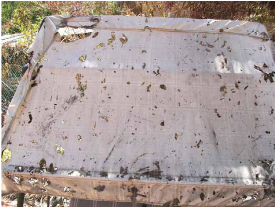
Figure 19 : This is the ember attack on a swing at the rear of a destroyed home in the Clifton Hills area.
