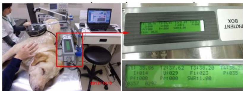
Figure 5. The patient box and its display during treatment
