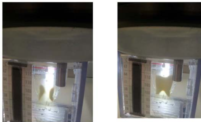
Figure 8. Coagulation of egg-white starts in its inner-volume, while the water around remains cold
