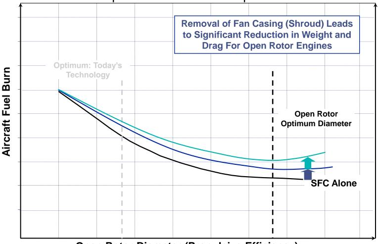
**Open Rotor Diameter (Propulsive Efficiency)**
