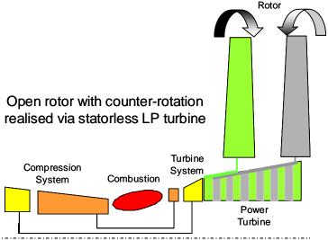
Statorless LP Turbine Design
