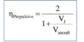
Propeller moves LARGE MASS of air at low velocity
