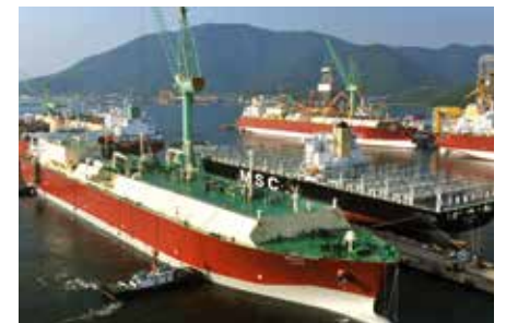
The Lloyd's Register classed Mozah , the first ever Q-max LNG carrier, an example of a membrane type gas ship.
