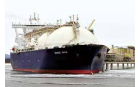
The Lloyd's Register classed Grand Aniva , an example of a Moss type gas ship.
