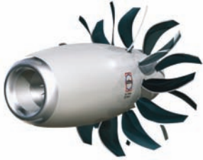
Snecma is heading up SAGE work on the direct-drive open rotor concept engine.
