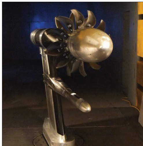
Increased wave drag can be obviated by increasing the number of blades and developing swept or scimitar designs.
