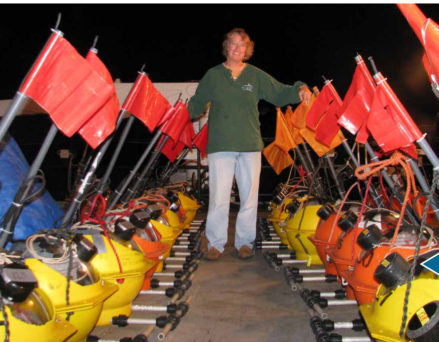
Gail standing in a fleet of ocean bottom seismometers ready for deployment in the Gulf of Mexico.
