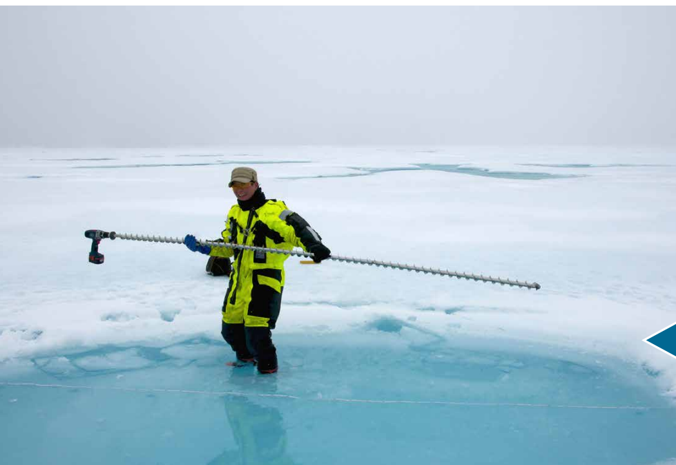
Drilling holes through sea ice—one of my favorite pastimes... And still essential for measuring sea ice thickness.
