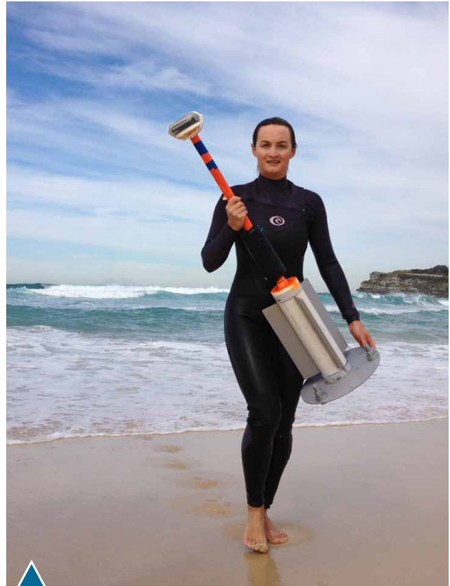
Kristen at Bondi Beach, NSW, Australia. She is carrying a drifter with a GPS that was being used to track currents as part of a rip current experiment.
