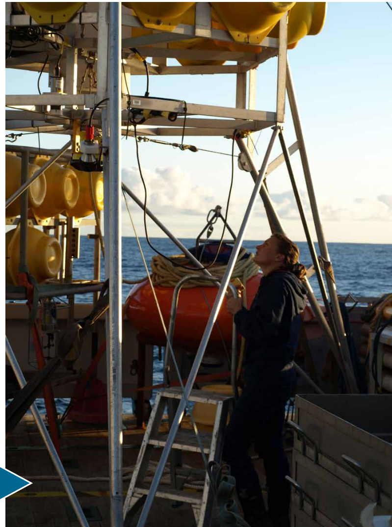
Preparing a bottom lander during a cruise on R/V Pelagia near Rockall Bank.
