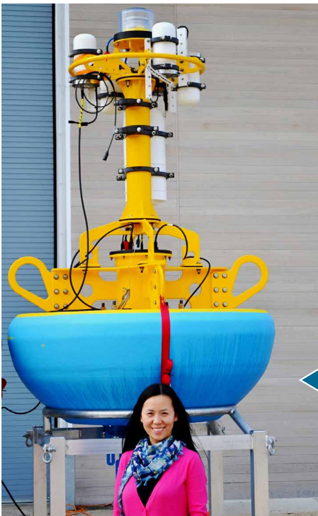
Xujing Jia Davis in front of a surface mooring at WHOI. One important part of her postdoctoral research is based on surface-mooring measurements in the Gulf Stream region.
