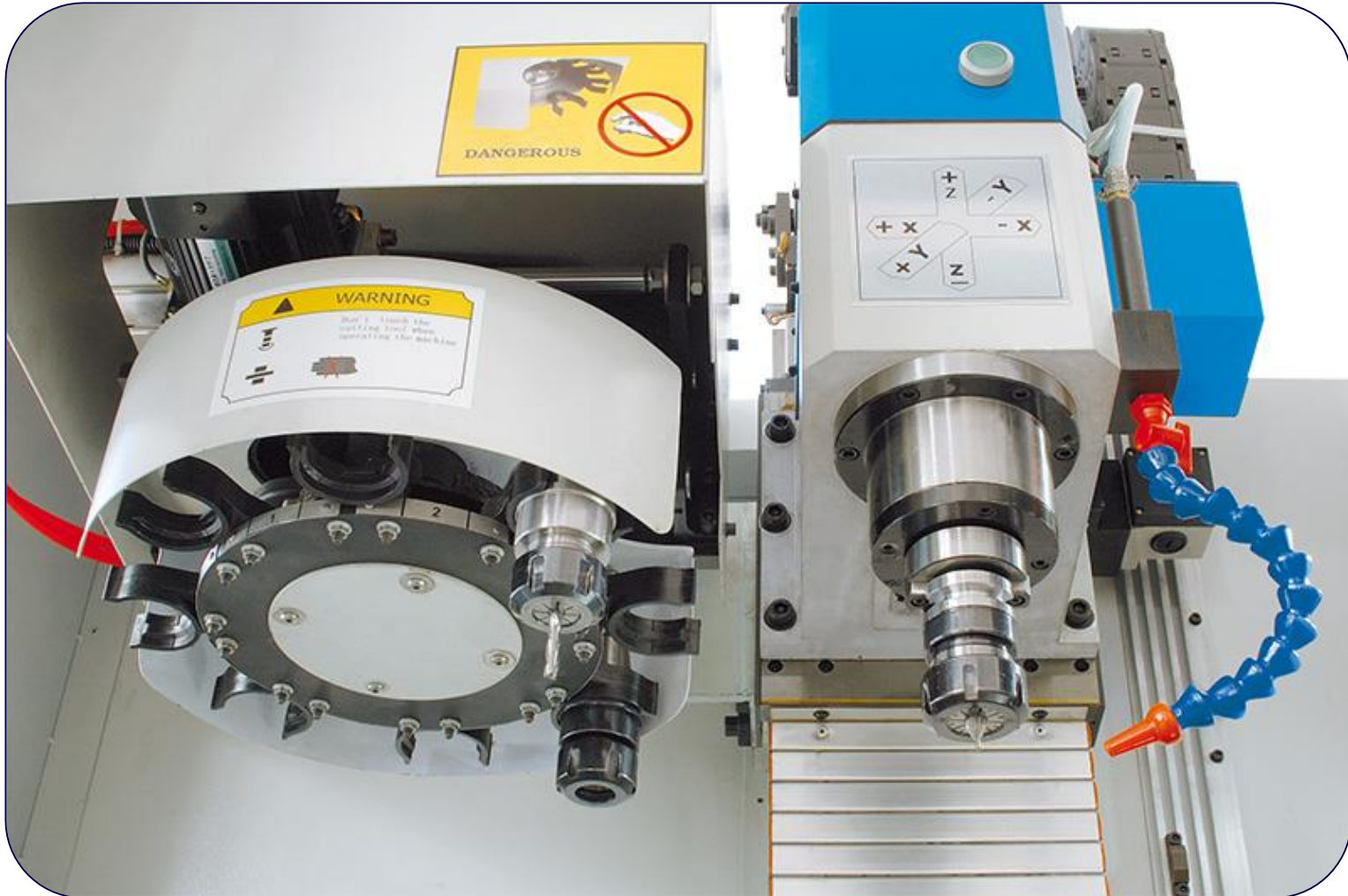
FIGURE 4-16: 8-station tool changer on a horizontal machining center
