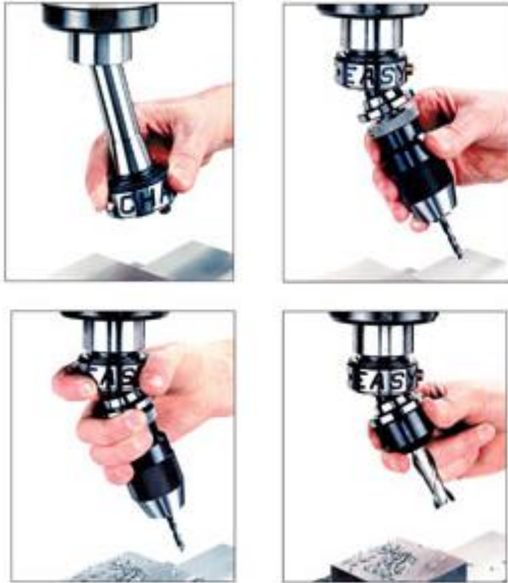
FIGURE 4-6 A quick change tooling system used for manual tool change
