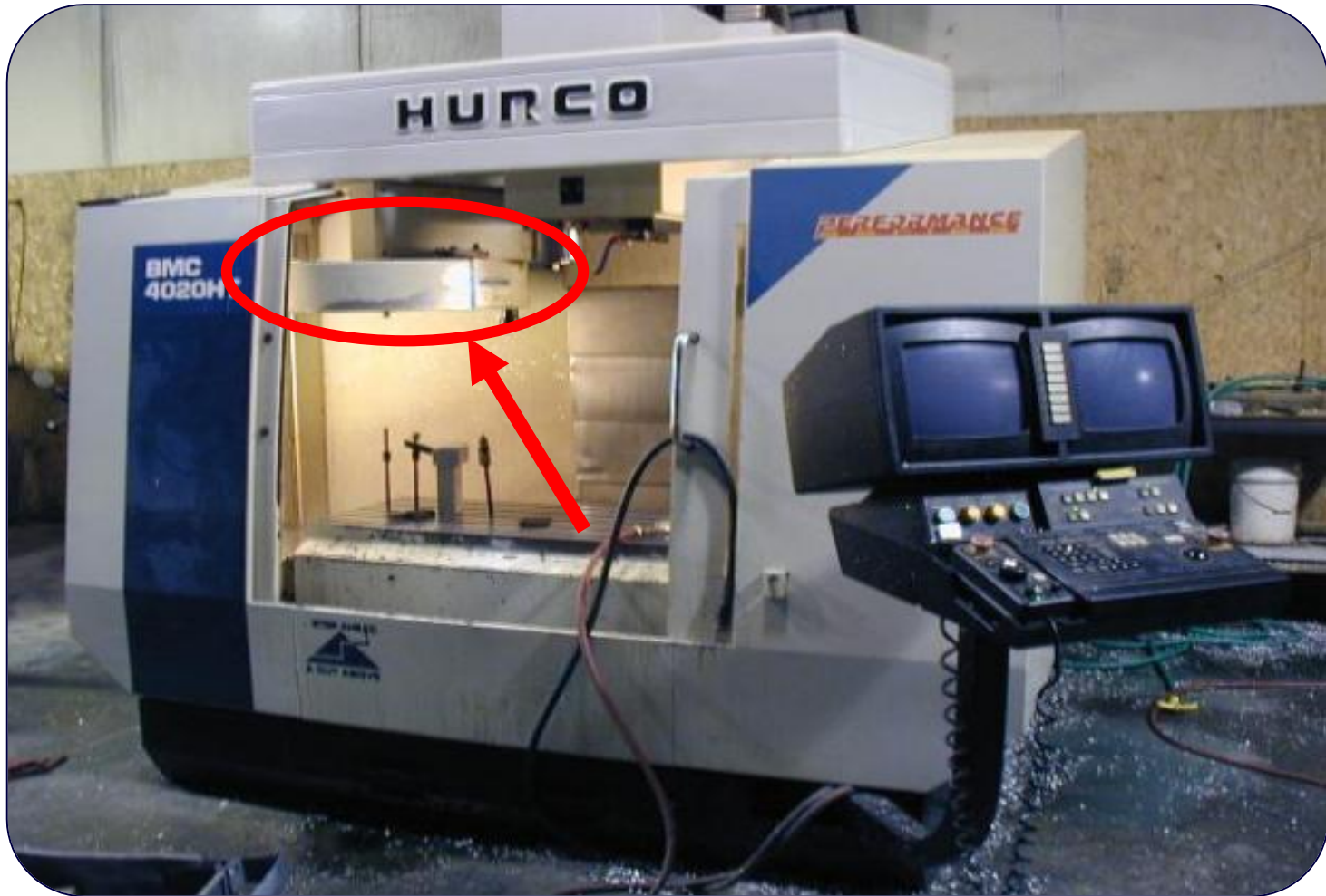
FIGURE 4-20: A vertical spindle machining center using carousel tool storage (Photo HURCO)
