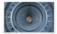
The specific design of the core end plates enables the stator core to be maintained under a constant axial pressure.
