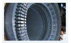
This structure is axially flexible to allow thermal expansion; it is also stiff in the radial and tangential directions to withstand high electromagnetic forces. The endwinding can easily be tightened during maintenance.
