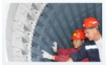
The use of Roebel bars for the duallayer stator windings minimises the eddy-current losses and maximises efficiency.
