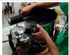
These photos are of the genset getting the final checkout before boxing it up to take to TARDEC. None of the components could be bought off the shelf, not the pumps, atomizing air compressor, coilstack, engine parts, feed pump, flat plate condensor/radiator, alternator. "Development" means most of these items were designed and tested and optimized and built again, several times.
