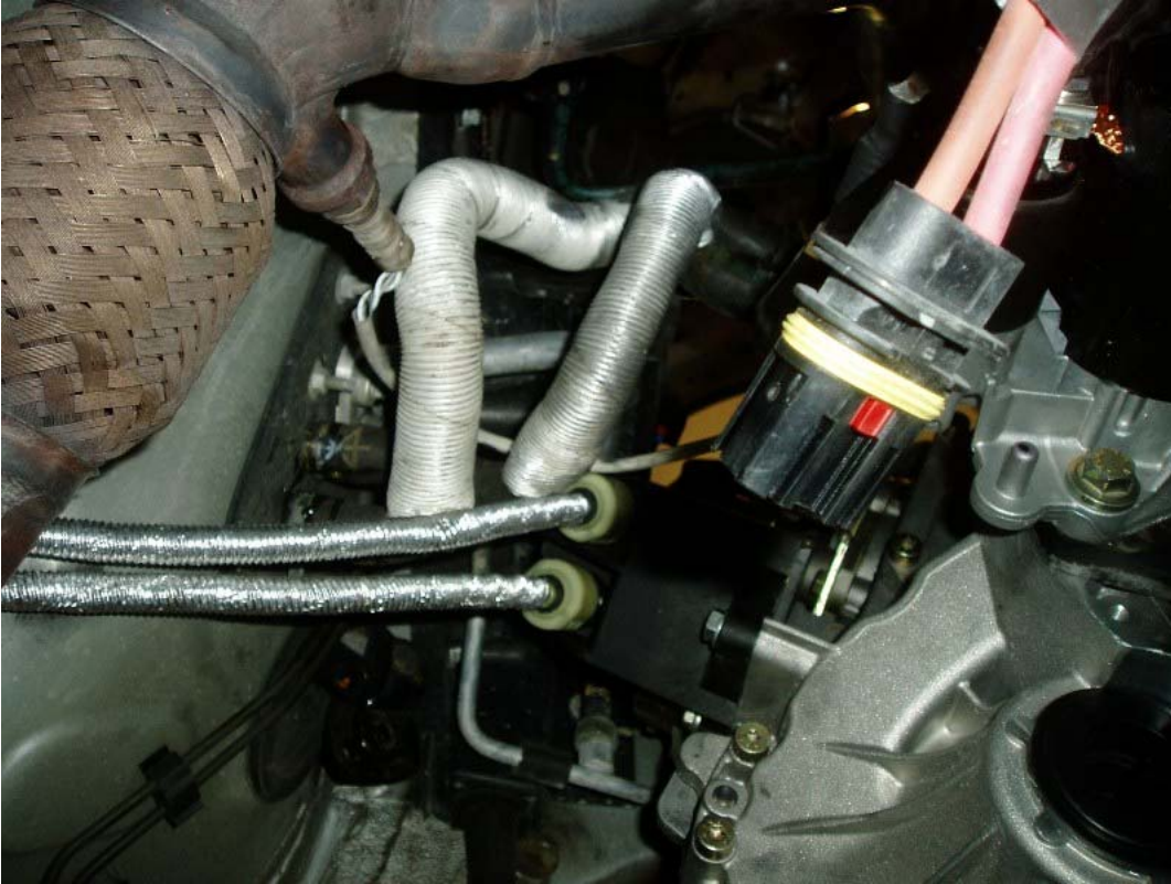
Figure 24 - Final shift cable routing.
