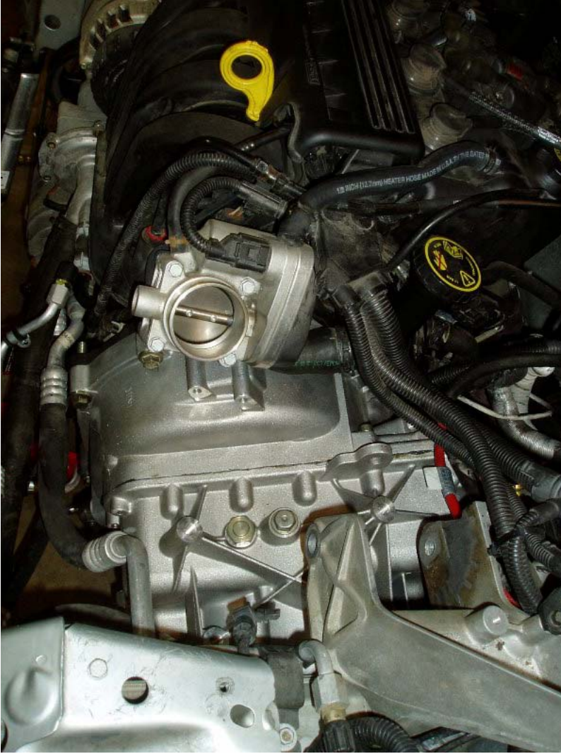
Figure 20 - Transmission bolted up, bolts torqued, ready to move on!
