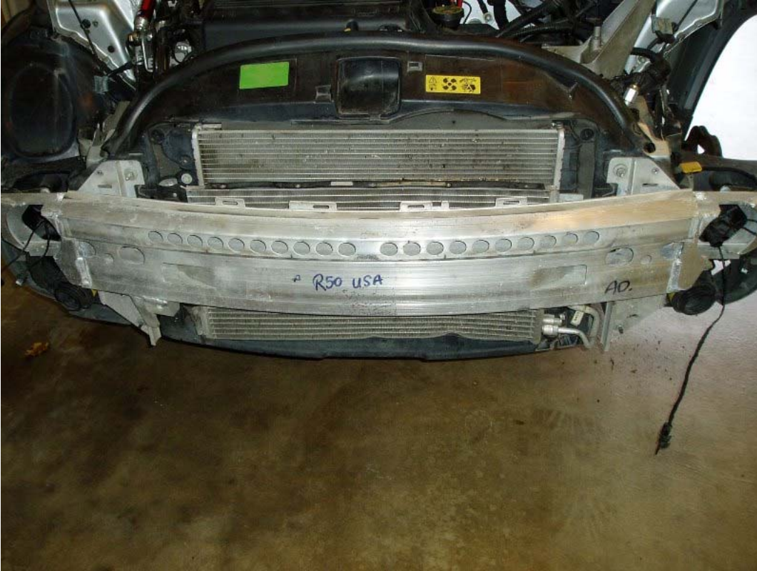
Figure 9 - Oooh, nekkid! Front bumper cover removed. And yes, the A/C condenser took some cone damage in the past.
