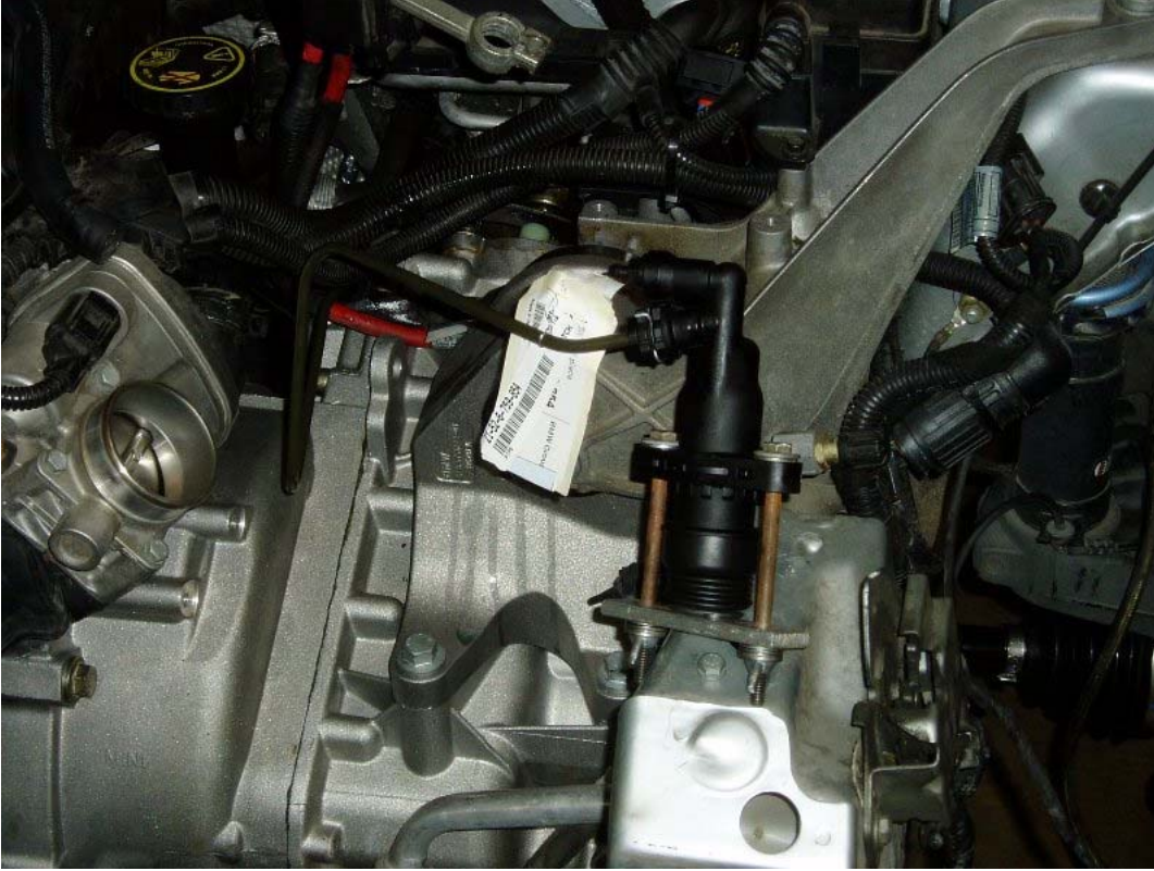
Figure 22 - New slave cylinder connected. Note the ghetto fabulous tool we made to keep the slave cylinder compressed for bleeding.
