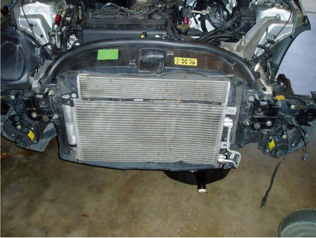
Figure 10 - Aluminum beam removed.
