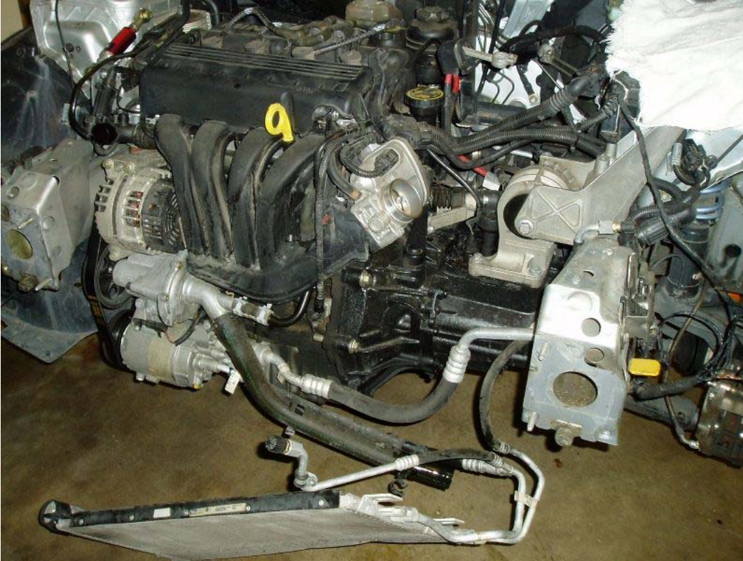
Figure 11 - Radiator core support and radiator removed.
