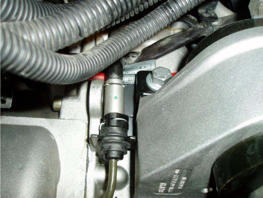
Figure 23 - Pipe bracket in place, securing the clutch line and pipe.
