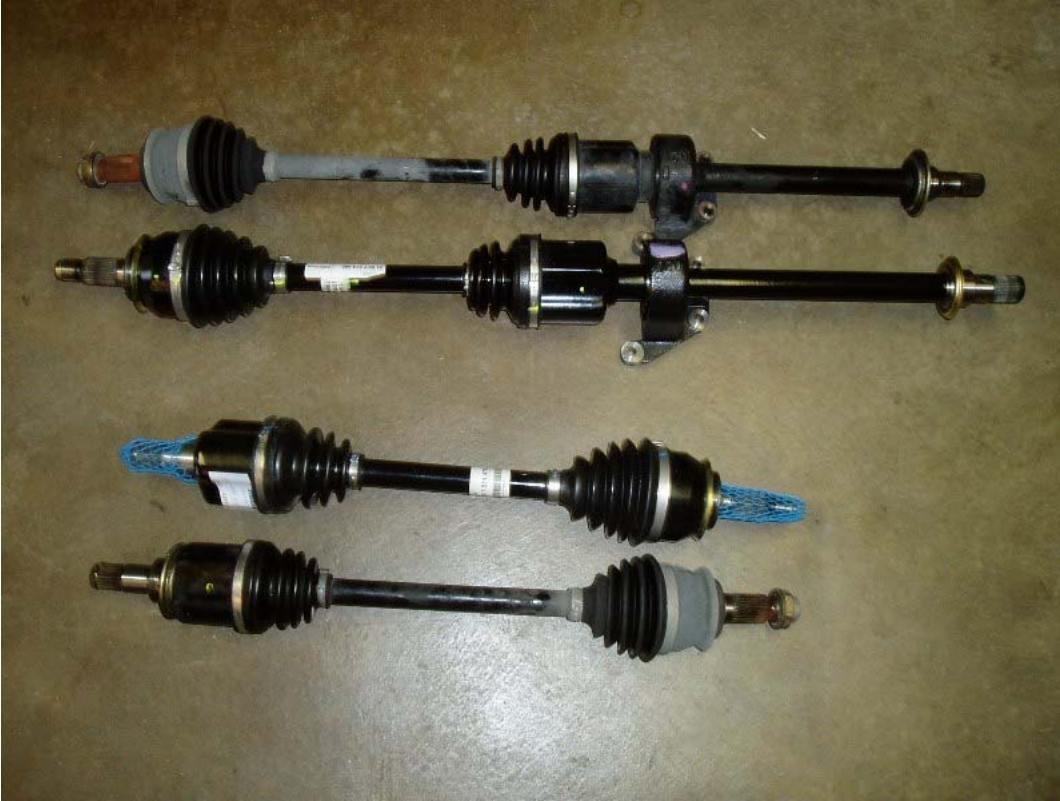
Figure 7 - Comparison of output shafts. The new shafts are obviously the clean ones - note that the passenger output shaft from the Cooper S has a longer prop shaft.
