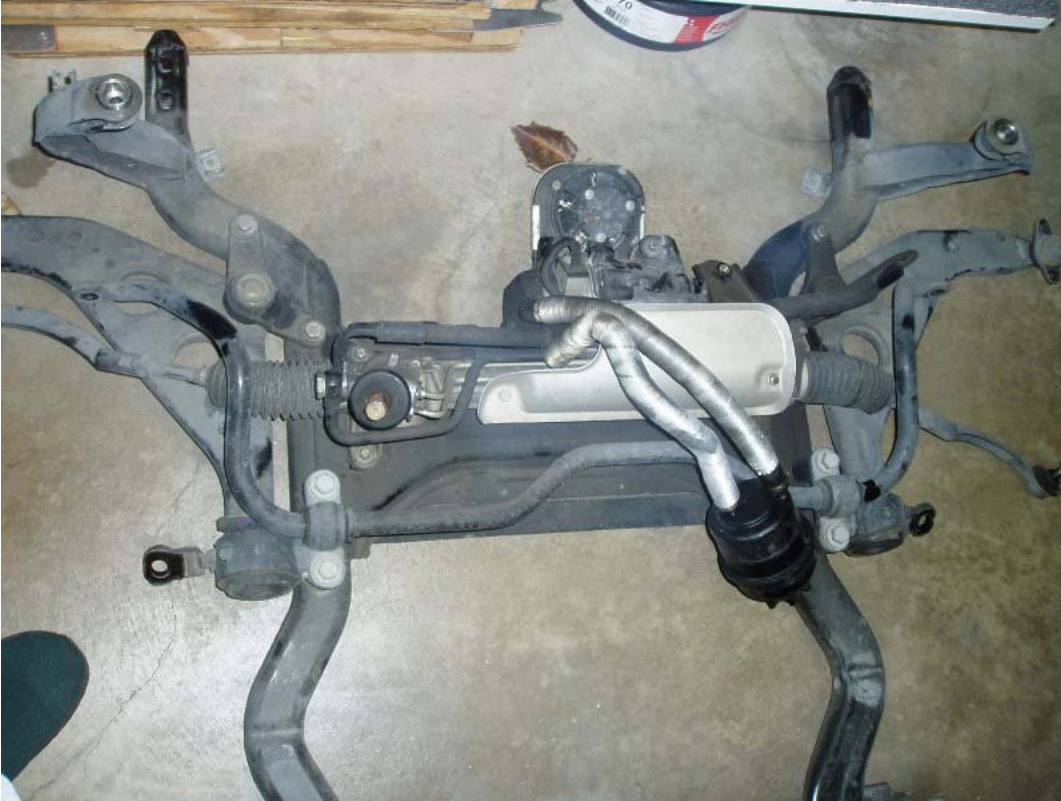
Figure 12 - Subframe removed and out of the way. Note this is before we rigged the power steering reservoir to remain upright using a stick and some duct tape.
