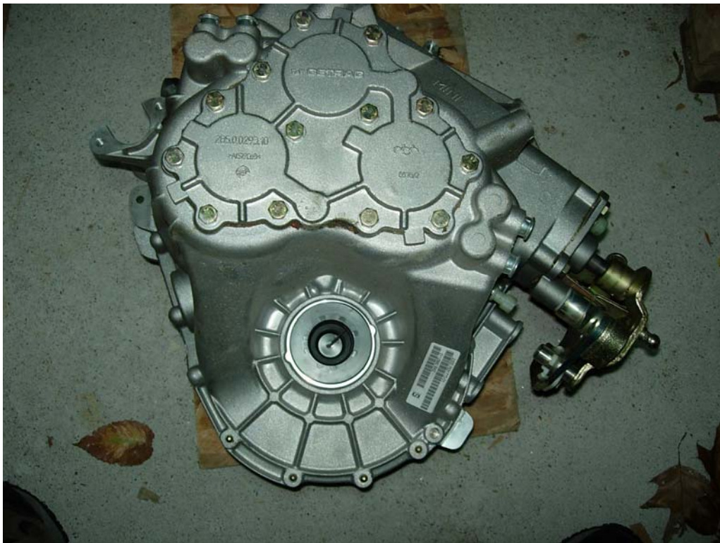
Figure 2 - Getrag 6-speed. Note the location of the part number sticker for reference. This is a brand new, never been used beauty!
