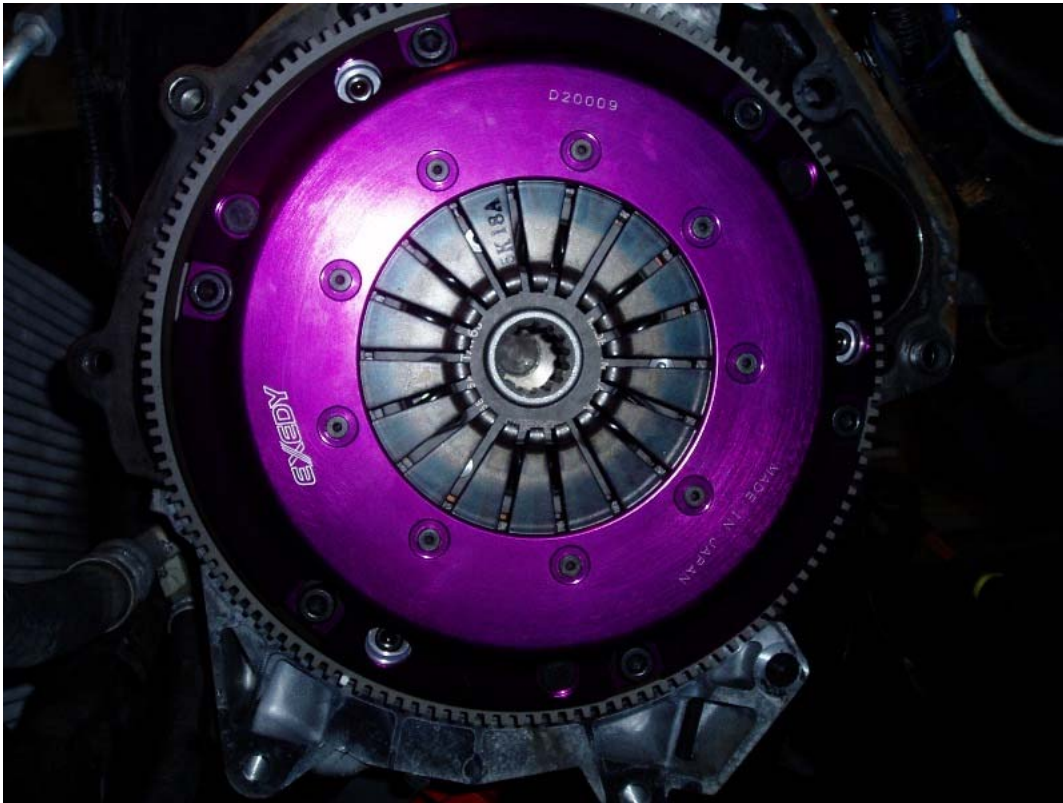
Figure 18 - Exedy Hyper Single flywheel, clutch and pressure plate installed. What a work of art - too bad nobody will ever see it! Note that the clutch disc is fairly well centered and ready to accept the input shaft from the new Getrag.
