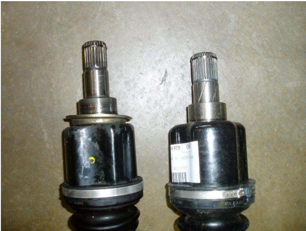
Figure 6 - Tranny side of the driver’s side output shafts - Cooper on the left, Cooper S on the right. Note the relief oiling in the Cooper S output shaft and more splines. Also note the missing dustcover - glad I ordered those!
