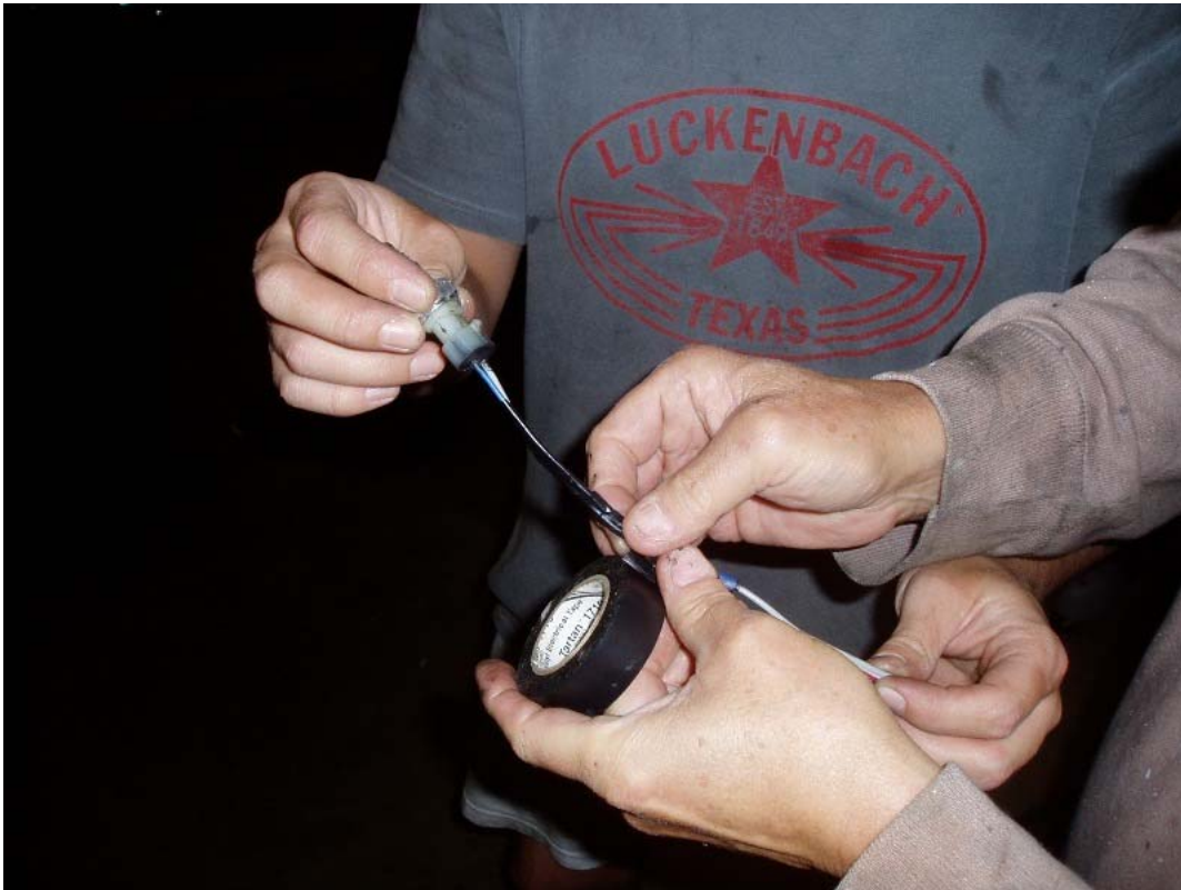
Figure 25 - Wrapping up the new backup light switch.
