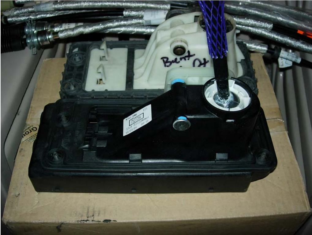
Figure 17 - Comparing the shift lugs. The white one is 'condition A' and the black one is 'condition B'. Use the one that matches your build date.
