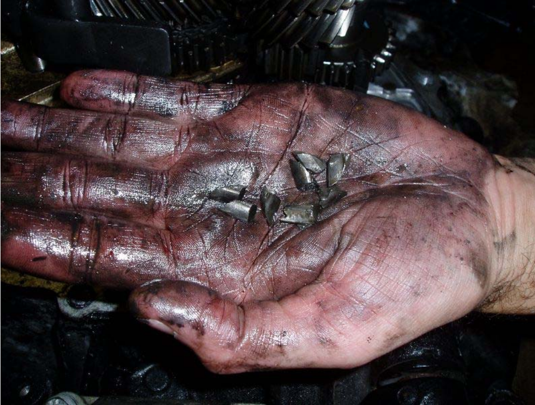
Figure 1 - Generally, this is not what you want to find inside your transmission.
