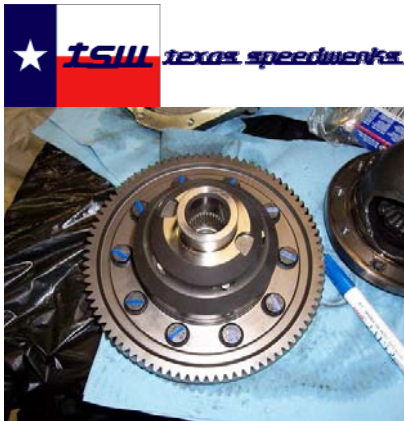
Figure 16 - Painted bolt heads, showing final location after torquing.
