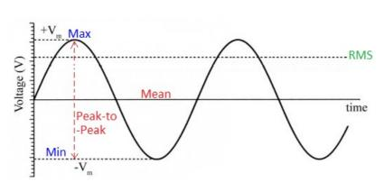
• RMS value of a sine wave = Peak Voltage /  $\sqrt{2}$
