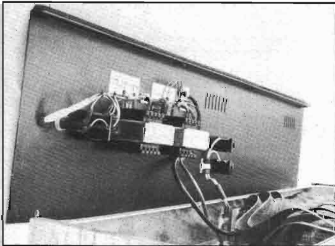
Above: prototype back panel. Production models may differ. Right: the voice boards plug directly into the mother board.
