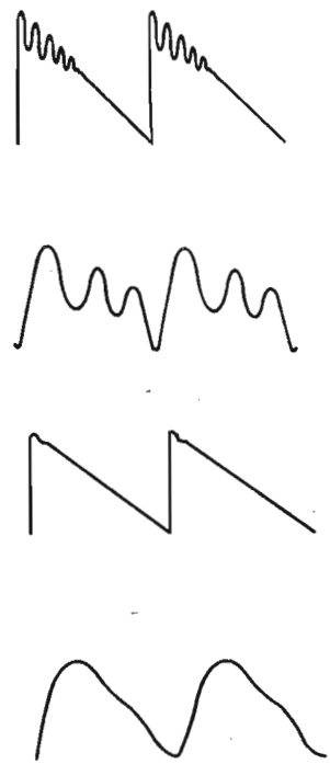
Fig.5 VCF response. From top to bottom: high frequency, high Q (resonance control clockwise); low frequency, high Q; high frequency, low Q (resonance control anticlockwise); low frequency, low Q.
