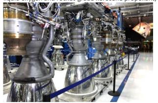
of thrust at liftoff, rising to 716 kilonewtons (161,000 pounds) as it climbs out of Earth's atmosphere. Merlin's thrust-to-weight ratio exceeds 150, making the Merlin the most efficient booster engine ever built, while still maintaining the structural and thermal safety margins needed to carry astronauts.
