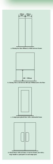
Note: An amendment to Part K of the Building Regulations, which came into effect in 1998, requires that swing doors should incorporate vision panels. See our leaflet on Regulations for Stairs, Ramps and Barriers for full details.
