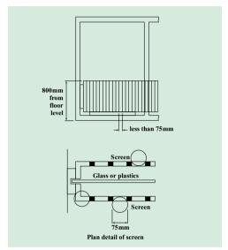
Figure 2. Permanent screen protection
