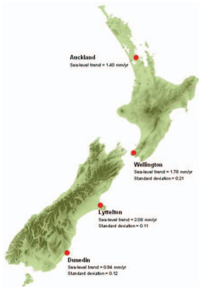
Figure 2.2: Linear trends in relative sea-level derived from New Zealand's four long-term port records for data up to 1998 (Dunedin), 2006 (Auckland) and 2001 (Wellington and Lyttelton). Corrections to mean annual sea level have been made for datum shifts, nodal tides (8.8- and 18.6-year tides) and annual pressure and temperature differences. The lower rate of rise for Dunedin is due to the low quality of the data and poor wharf stability, so less weight is given to this value in deriving the New Zealand average rate of rise. Sources: Hannah 2004; NIWA (for the update to 2006 for Auckland).
