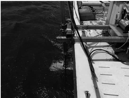
Fig. 3 (left) Multibeam sonar (SeaBat 8125) equipped with boat. (Y. Matsumoto)
