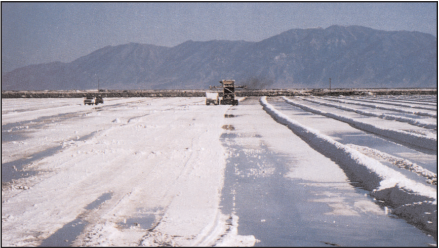
Harvesting potassium-bearing salts from large solar-evaporation pond. Salts will be processed into potassium sulfate, a mineral fertilizer.
