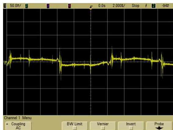
Fig-4: Output noise of "PZA" 1pc Vp-p=81mV
