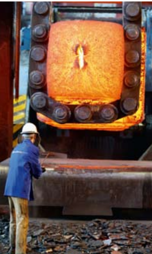
Forging grade ingot on 55 MN open-die forging press
