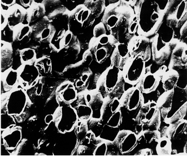
Fig. 16: Magnification of a separator, scale 500: 1 [3]
