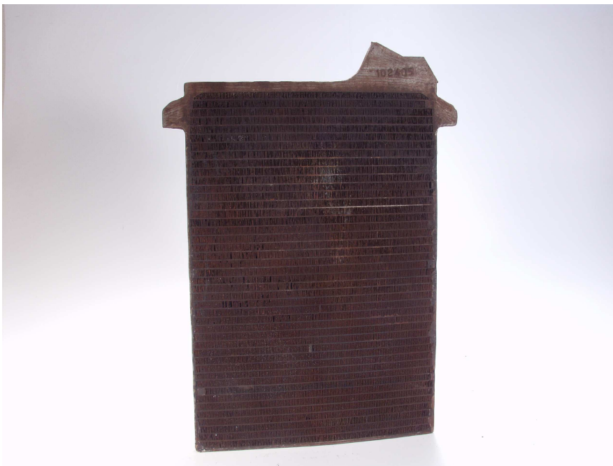
Fig. 10: Formed positive Planté plate
