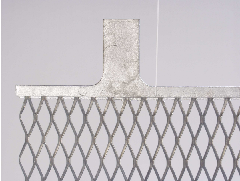
Fig. 15: Lead coated copper grid
