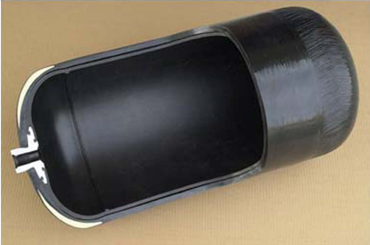
Figure 6. Plastic-lined stress rupture test vessel.
