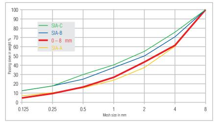
Fig. 25: dry sprayed concrete grading curve
