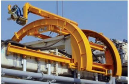
Fig. 11: TBM-spraying robot with telescoping spraying boom
