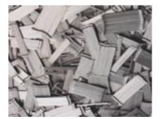
Fig. 19: steel fibres
