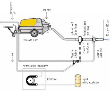
Fig. 39: dense-flow process for wet sprayed concrete
