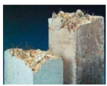
Fig. 18: failure surface of two prisms
