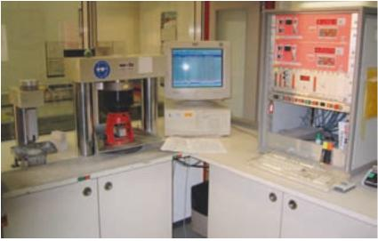
Fig. 37: core compression testing
