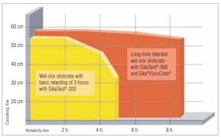
Fig. 15: Workability time of wet sprayed concrete mixes
