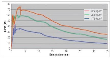
Fig. 20: plate test SIA 162/6, Steel fibre Dramix RC-65/35-BN
