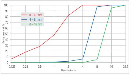
Fig. 12: Particle size distribution of individual components
