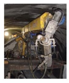
Fig. 47: Spraying robot with telescoping boom on the tunnel boring machine Karahnjukar in Iceland
