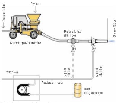
Fig. 51: thin-flow process for dry sprayed concrete
