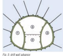
preceding drift walls (1, 2), followed by excavation of the crown 3) then the bench and invert (4) including
