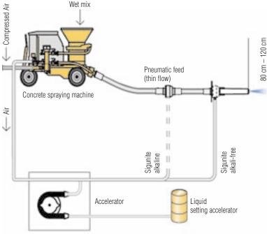
Fig. 40: thin-flow process for wet sprayed concrete
