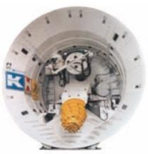
Fig. 7: shield heading machine operated by the joint venture for the Munich underground rail network, package U2, with spray manipulator moved upwards as additional stabilisation system
