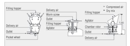
Fig. 50: operating principles of the two-chamber type machine, the screw-type machine and the rotor-typ machine
