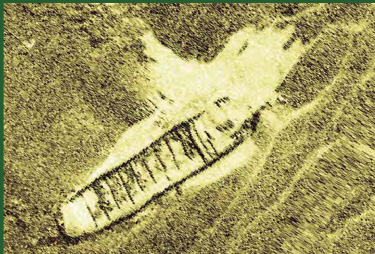
An example of a side-scan survey image of an 'anomaly', probably a wreck, measuring 41 x 15 metres, and 2.7 metres high
