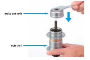
13. Screw on the stop nut to adjust so that the hub shell can be turned smoothly without any play. After adjusting, secure the stop nut with the left hand lock nut.
