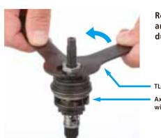
Remove the right hand lock nut and the right hand cone with dust seal from the hub axle.
