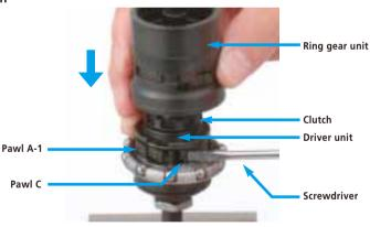
Turn the ring gear to the left and right while pushing down on the sprocket and check that it has an angle of play of approximately 10°.
