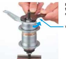
Remove the left hand lock nut from the hub axle, and then remove the stop nut.
