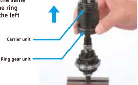
After removing them at the same time, remove the carrier unit from the ring gear unit.
