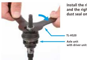
Install the right hand lock nut and the right hand cone with dust seal onto the hub axle.
