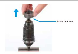
6. Remove the stop ring with a screwdriver. At this time, the stop ring come off with great force. Be careful of the safety using cloth and so on.
