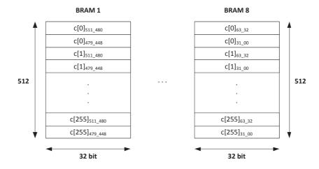
Fig. 3. Our smallest table based FPGA implementation of RFSB-509 requires 8 block memories configured as  $512 \times 32$  bit dual-port ROM. Every BRAM holds a 64-bit chunk of the 509-bit constants (prepended by three zero bits) split into two 32-bit parts. Since two memory slots of each BRAM can be read out in one clock cycle, one constant can be read out in one clock cycle.
