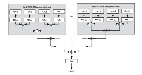
**Fig. 2.** The basic compression unit in RFSB consists of looking up four constants, rotating them according to their position by either 384, 256, 128, or 0 bits and xoring the result. The *fold* unit represents the reduction modulo  $x^{509} - 1$  by folding the three most significant bits onto the three least significant bits.
