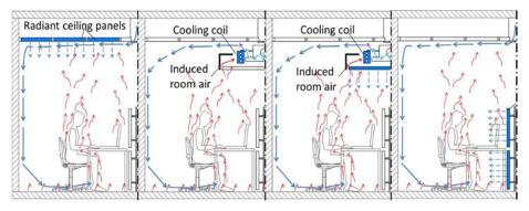
versus convection 50%). With chilled beam as with allair systems, heat transfer is only based on convection.
