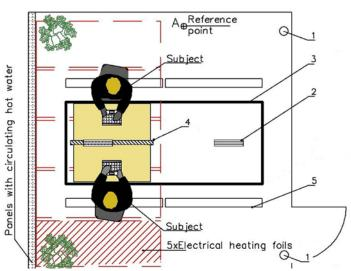
**Figure 2.** A) Top view of the test room with measurement pole locations: 1) ventilation exhaust, 2) ventilation supply, 3) chilled beam (CB), 4) desk partition mounted radiant cooling panels, 5) light fixtures, B) photograph of the measurement setup in CB, CBR and CCMV cases and C) photograph of the measurement setup in MVRC case (thermal mannequins above were used in actual measurements).
