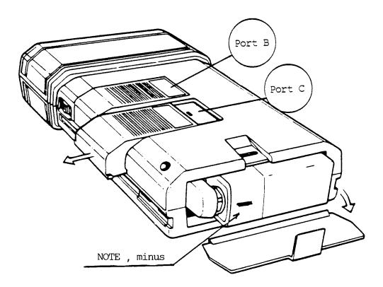
To connect the battery, slide it into the opening, making sure that the smaller, positive, terminal enters first. If the battery only slides in half way, then you have tried to put it in the wrong way round. Turn the battery over so that the other metal contact slides into the battery connector first, and try again.
